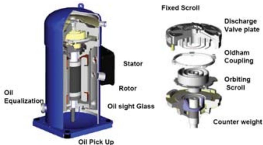
Figure 88. Compressor Internal Components, 15-30T
