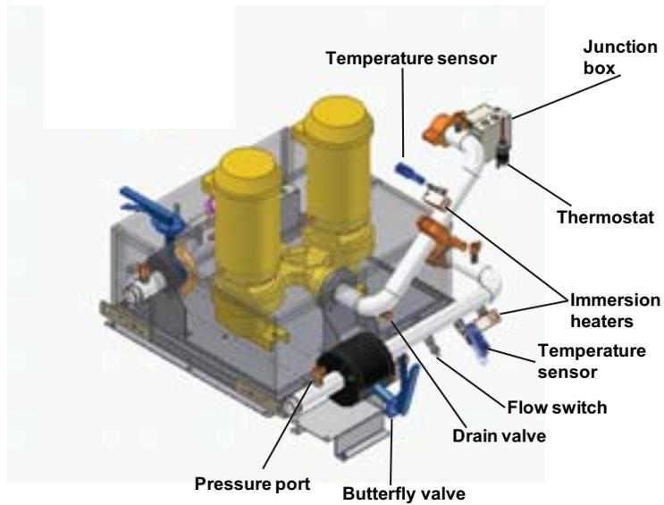
Figure 75. Pump package components, V40-70T, view 1
