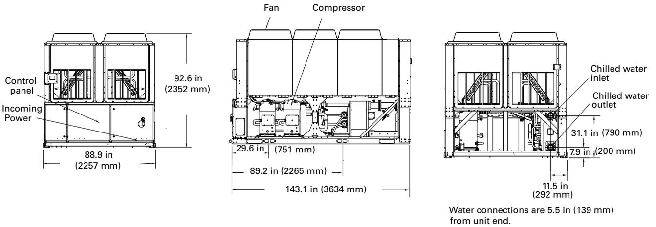
**Note:** When facing the control panel, circuit 1 is on the right side of unit.
