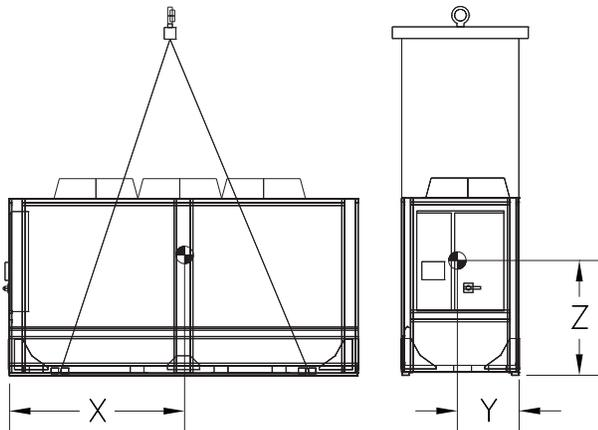
**Figure 36. CGAM V 40-70 Ton Rigging**
