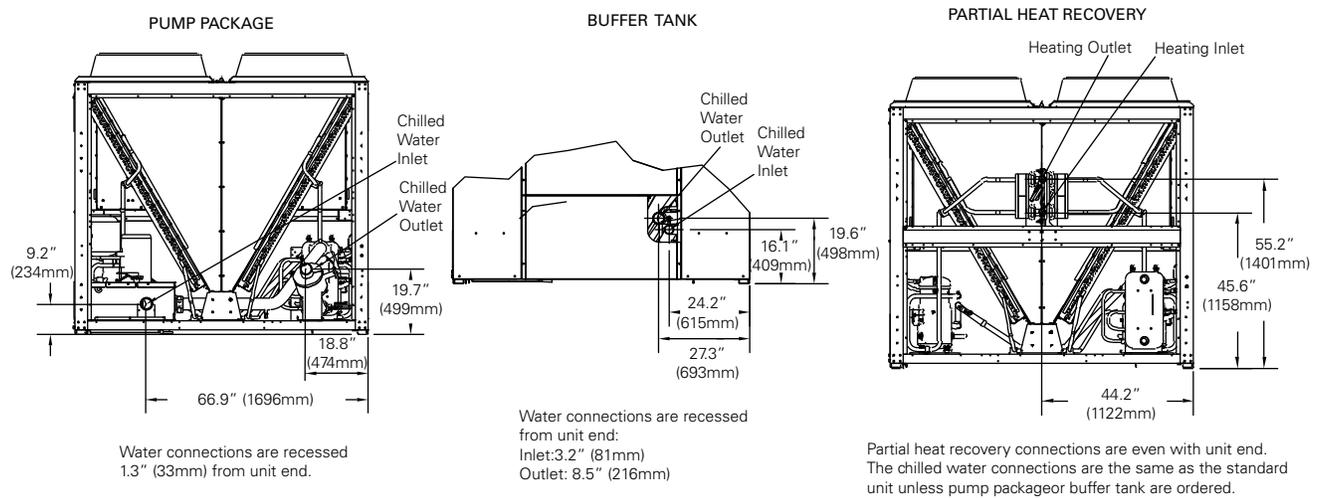
**Figure 33. CGAM 80 -130 ton — pump package, buffer tank, partial heat recovery unit water connections<sup>(a)</sup>**
