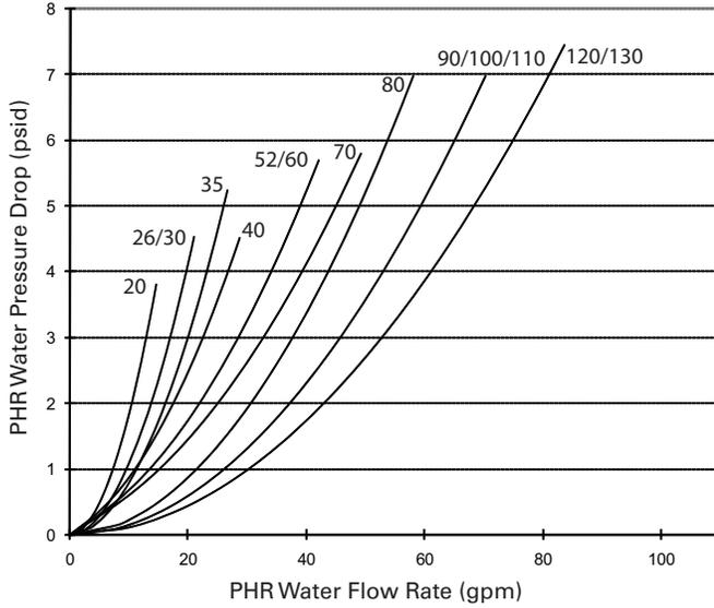
**Figure 58. Partial heat recovery pressure drop curve — 50 Hz**
