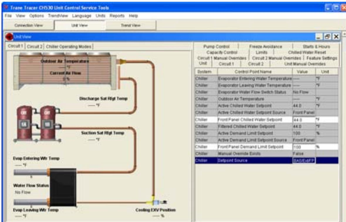
UnitView also displays, in real time, all non-setpoint data organized by tabs. As data changes on the chiller it is automatically updated in the Unit View.
