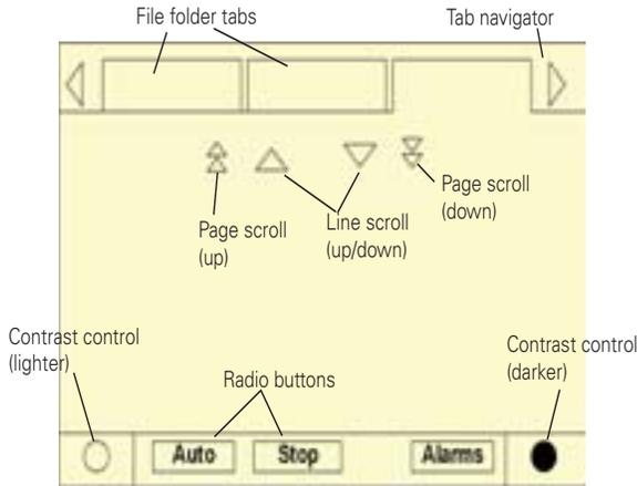
The file folder tabs across the top of the screen are used to select the various display screens.
