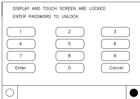
If the Display and Touch Screen Lock feature is Disabled, a similar screen including "Enter 159 to Unlock" will show if the MP temperature is approximately less than 32°F (0°C) and it has been 30 minutes after the last key stroke. Note: the main processor is equipped with an on-board temp sensor which enables the ice protection feature (OAT is not required).
