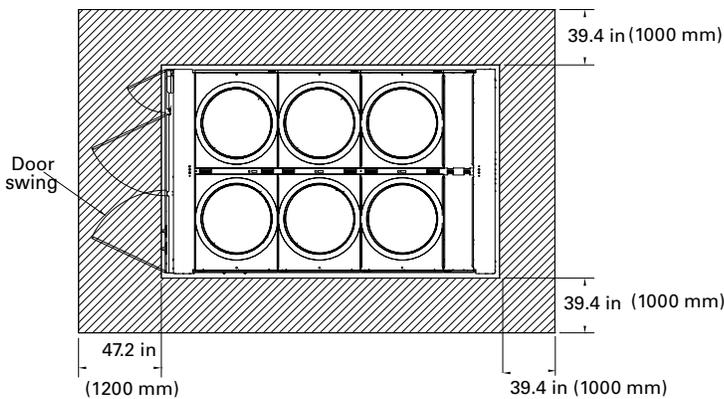
More clearance may be needed for airflow depending on the installation.
