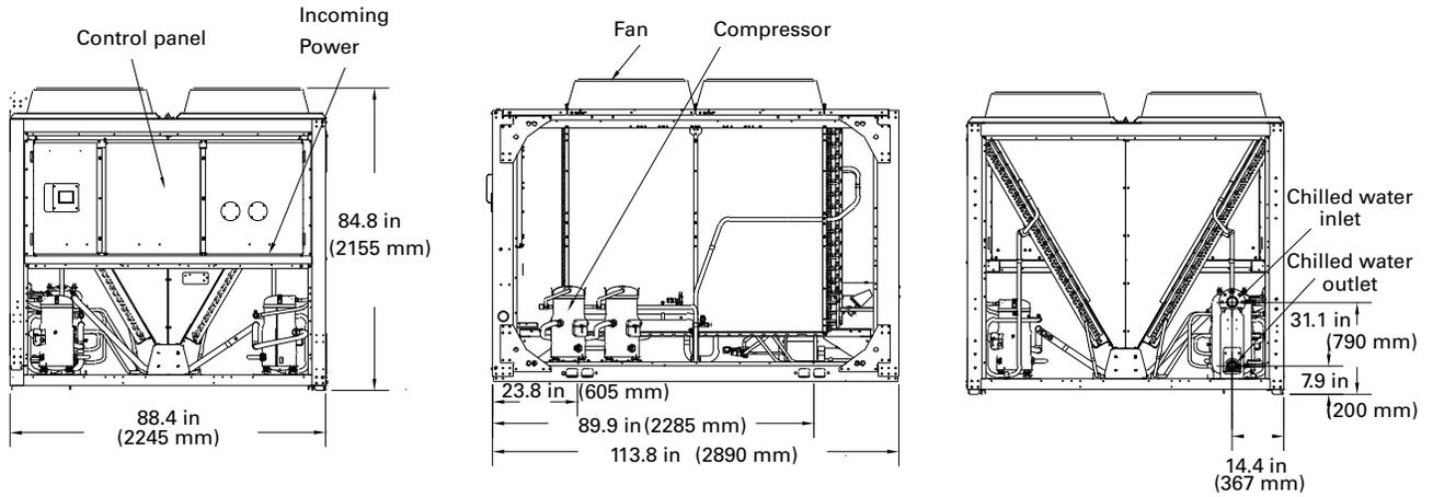
Water connections are even with unit end.
