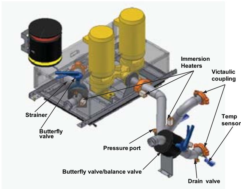
**Figure 77. Pump package components – V 40-70 ton – view 3**
