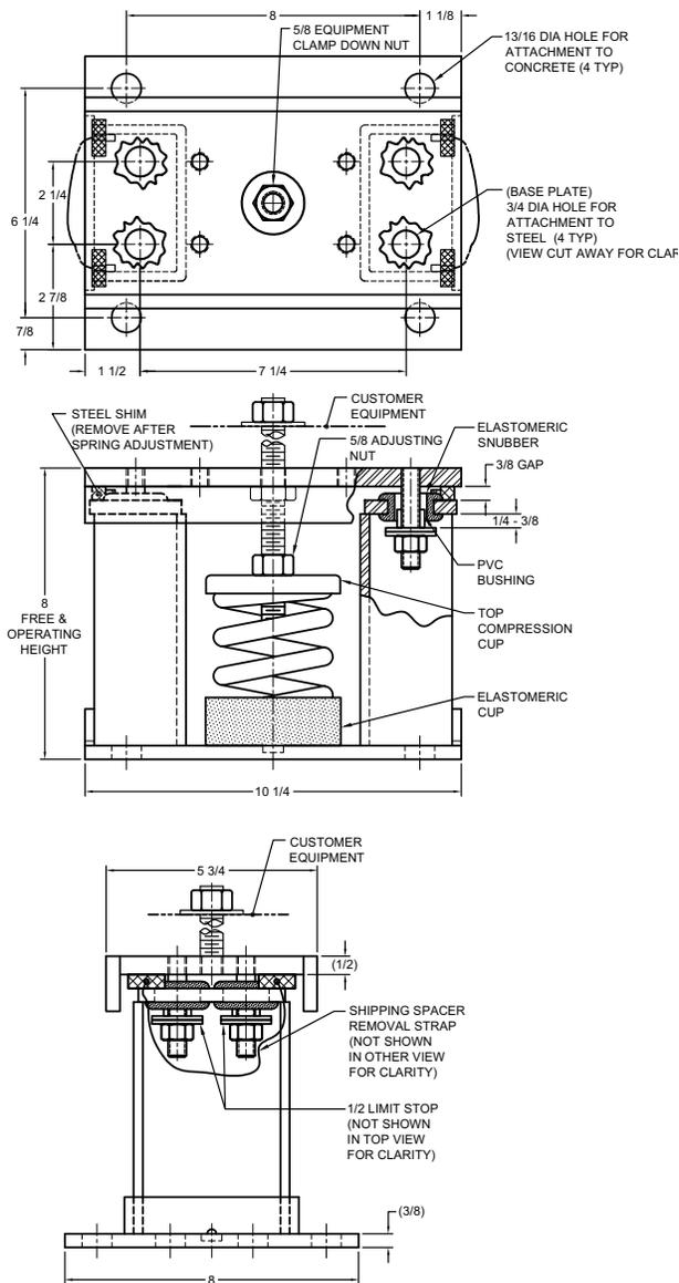
**Figure 40. M2SS seismically rated isolator**
