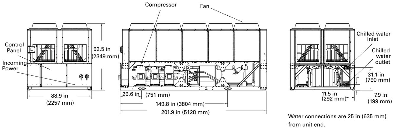
**Note:** When facing the control panel, circuit 1 is on the right side of unit.
