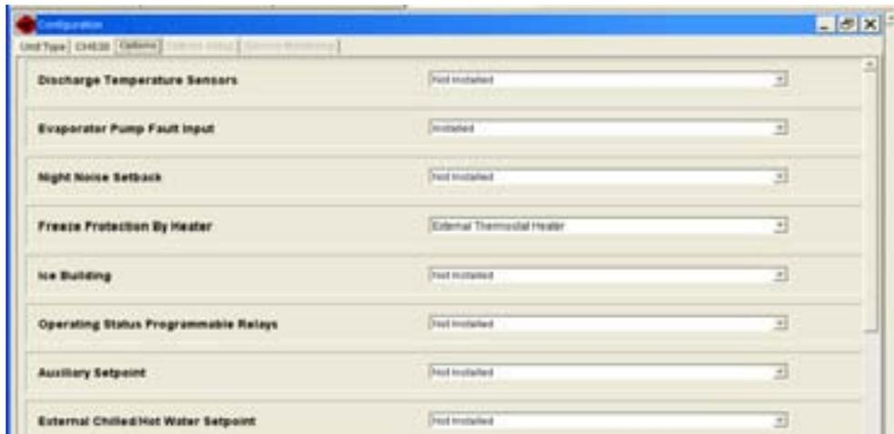
Figure 98. Configuration view - options setup tab
