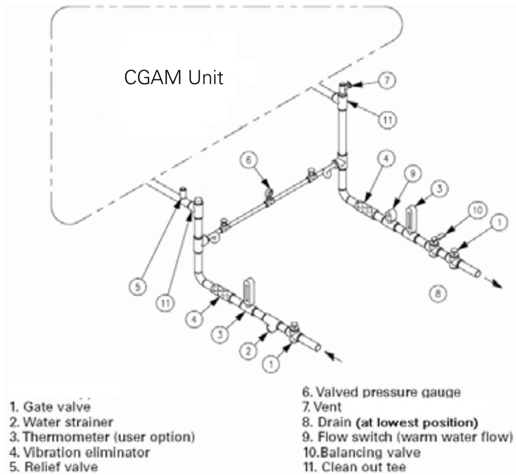
**Note:** In addition to those recommended for field piping, the CGAM unit includes factory installed manual air vent and water drain valve with partial heat recovery option. See [Figure 81, p. 96](#) through [Figure 83, p. 97](#) for partial heat recovery component locations.
