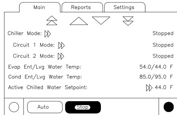
The Main screen shall be the default screen. After an idle time of 30 minutes the CH530 shall display the Main screen with the first data fields.
