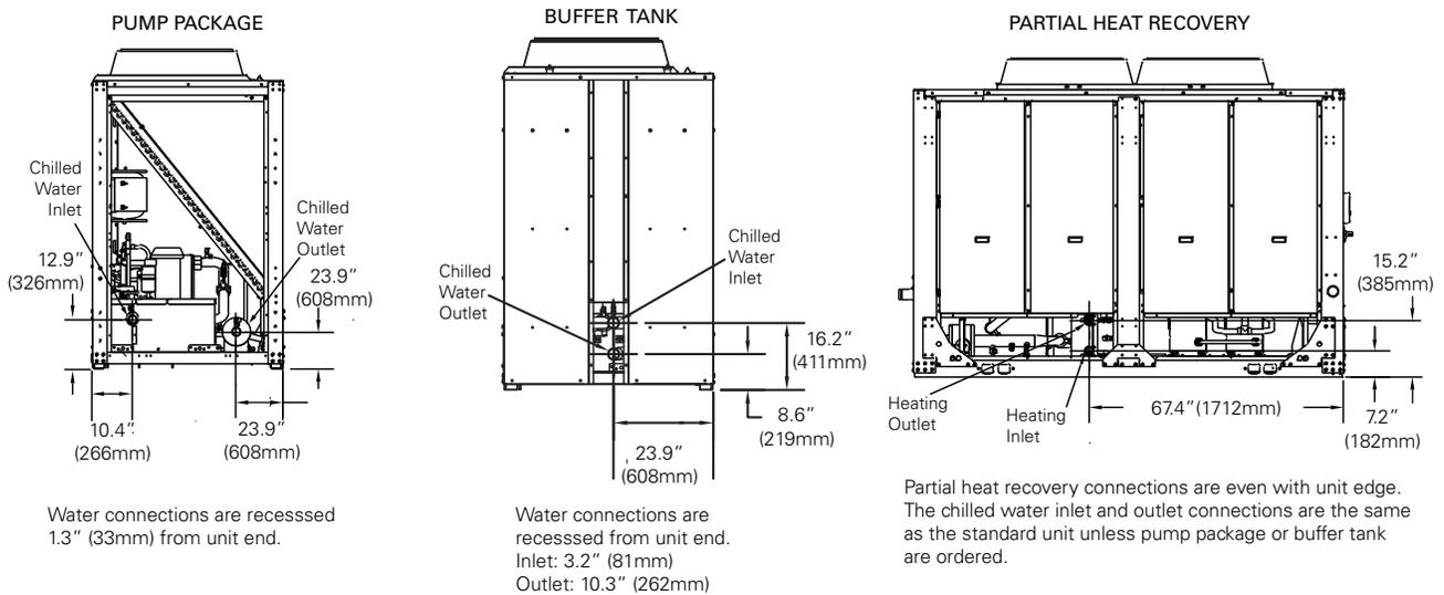
**Figure 31. CGAM 40 and 52 ton — pump package, buffer tank, partial heat recovery unit water connections**
