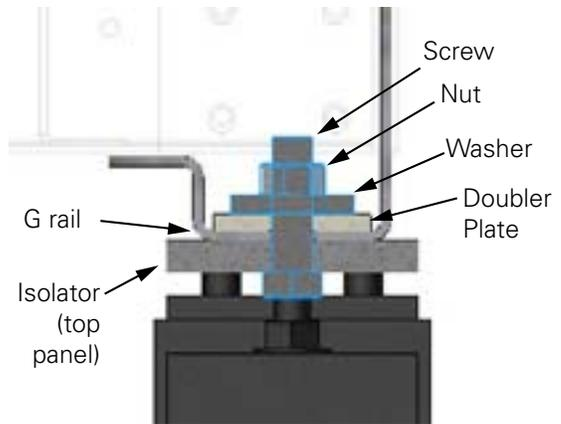
**Important:** The following adjustment process can only begin after the equipment or machine is at its full operating weight.
