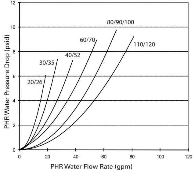
**Table 24. Partial heat recovery flow rates — 60 Hz**
