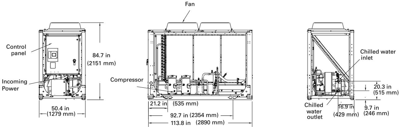
Water connections are 1.7 in (44 mm) from the end.
