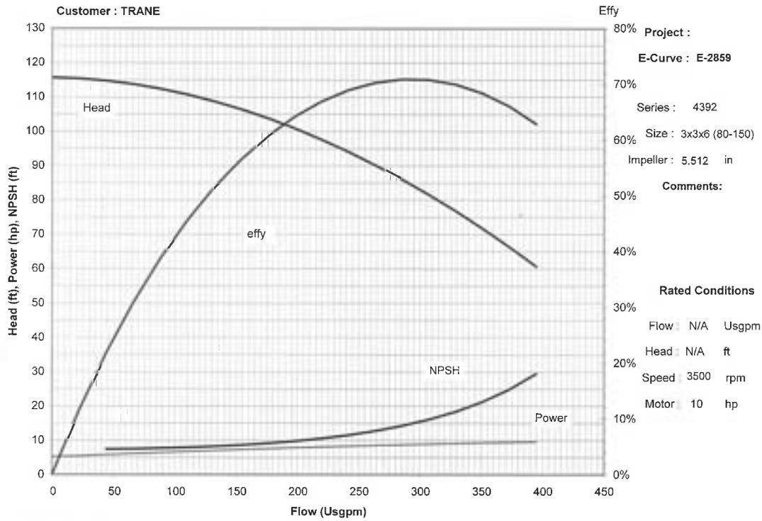
**Figure 64. Pump curve - 120-130T - water only**
