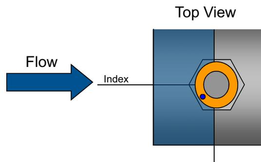
The flow switch must have the dot in the shaded area to the left of this line for proper indexing ( $\pm 90^\circ$  off Index)
