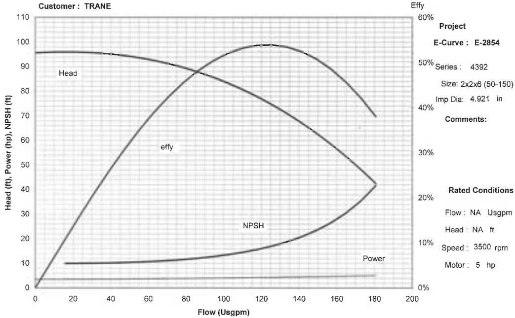
Figure 62. Pump curve - 60-70T - water only
