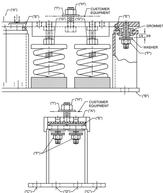
1. Set isolators on mounting surface, ensuring that all isolator centerlines match the submittal drawing. All isolator base plates (B) must be installed on a level surface. Shim or grout as required, leveling all isolator or base plates at the same elevation.
