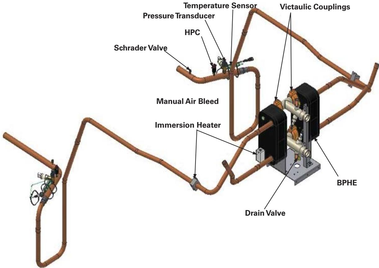
Figure 83. Partial heat recovery components — W 80-130 ton
