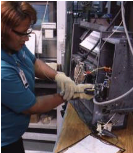
Figure 4: Fan-coil During End-of-Line Testing
