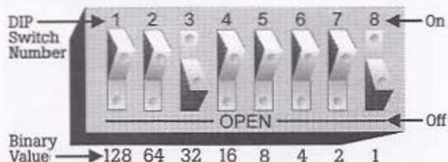
2. Short and hold the test input until all LEDs are on. Then, remove the test input signal. Figure 19 shows an example of the test input. Use a coin or other object to short the test input. Or, set the DIP switches with power off to the TUC, then apply power. The TUC will read the DIP switches at power up (Rev 12 TUC or higher).
