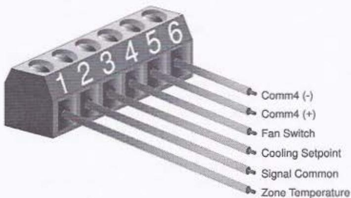
**Figure 11** Connections for a 2-wire Terminal Block
