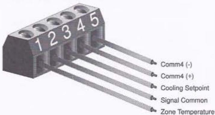
**Figure 10** Connections for a 6-wire Terminal Block
