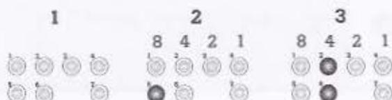
**Sequence 1** shows all LEDs off. When you short and hold the test input, all LEDs go off for one second.
