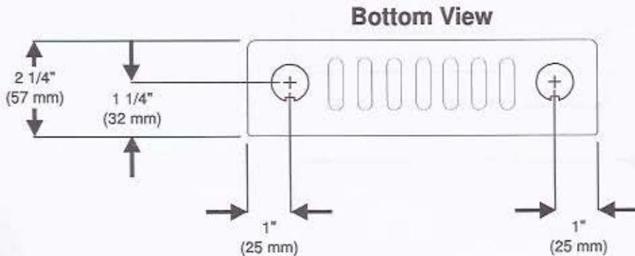
Figure 5 Dimensions of the Resin Enclosure
