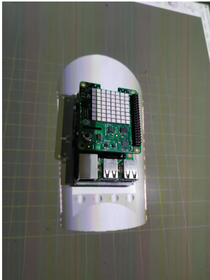
This picture highlights a project of rising eighth graders Noah Warren and Bud Gidiere who are working on a wearable computer. They are designing a 3D print to attach the computer, which is a Raspberry Pi, to their arm.
