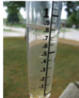
Rain Gauge Measures amount of precipitation
