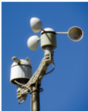
Anemometer Measures wind speed
