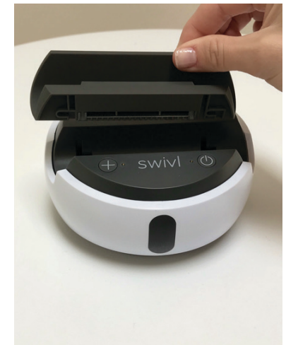
4. Align the grip back in the grooves of the base and slide it to the right
