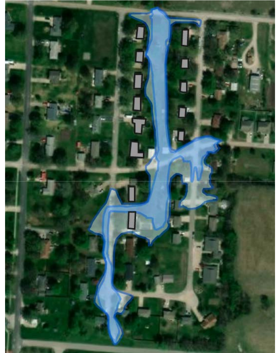
ES&S – Calculated 100-year Floodplain with 25-year Storm Sewer Pipes
