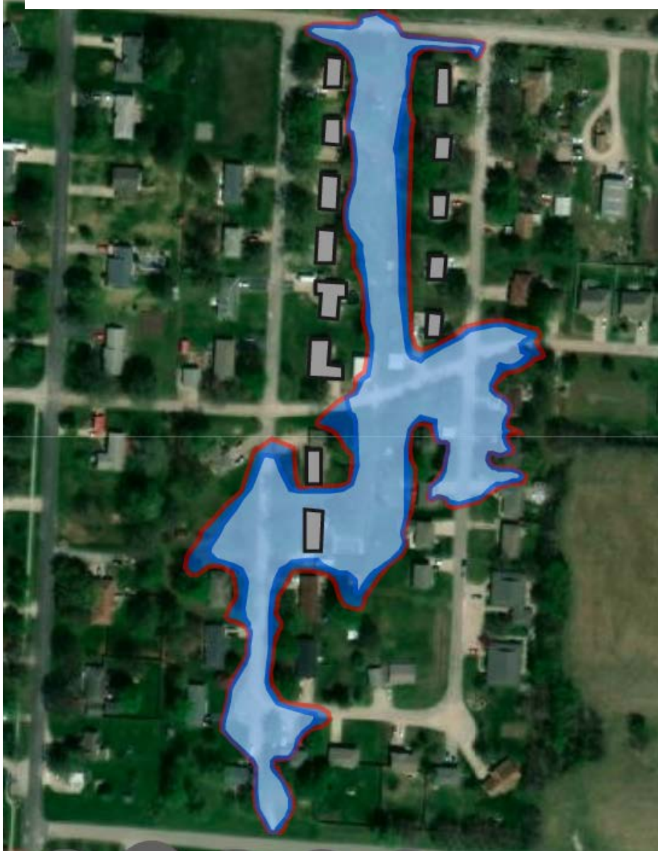
ES&S – Calculated 100-year Floodplain with 10-year Storm Sewer Pipes
