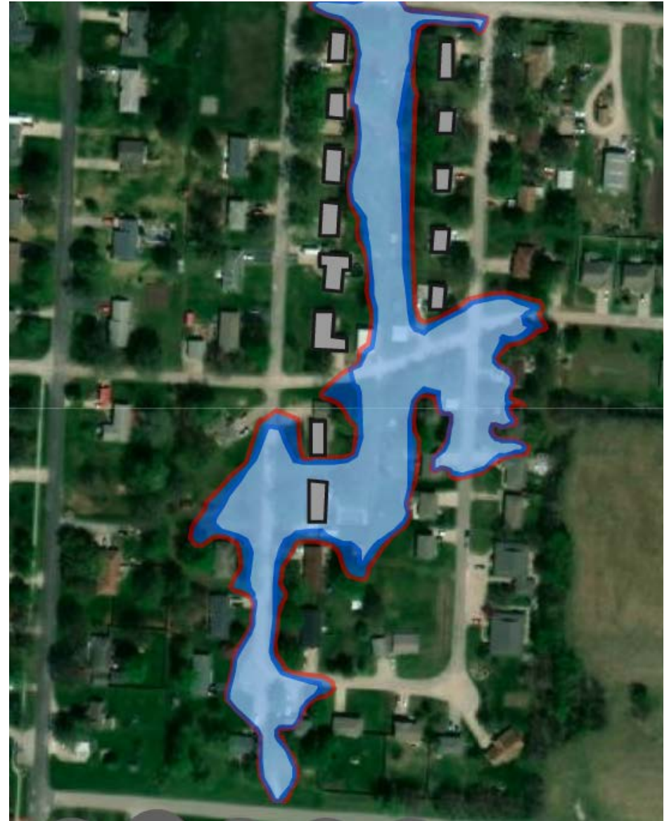
ES&S – Calculated 100-year Floodplain with 10-year Storm Sewer Pipes
