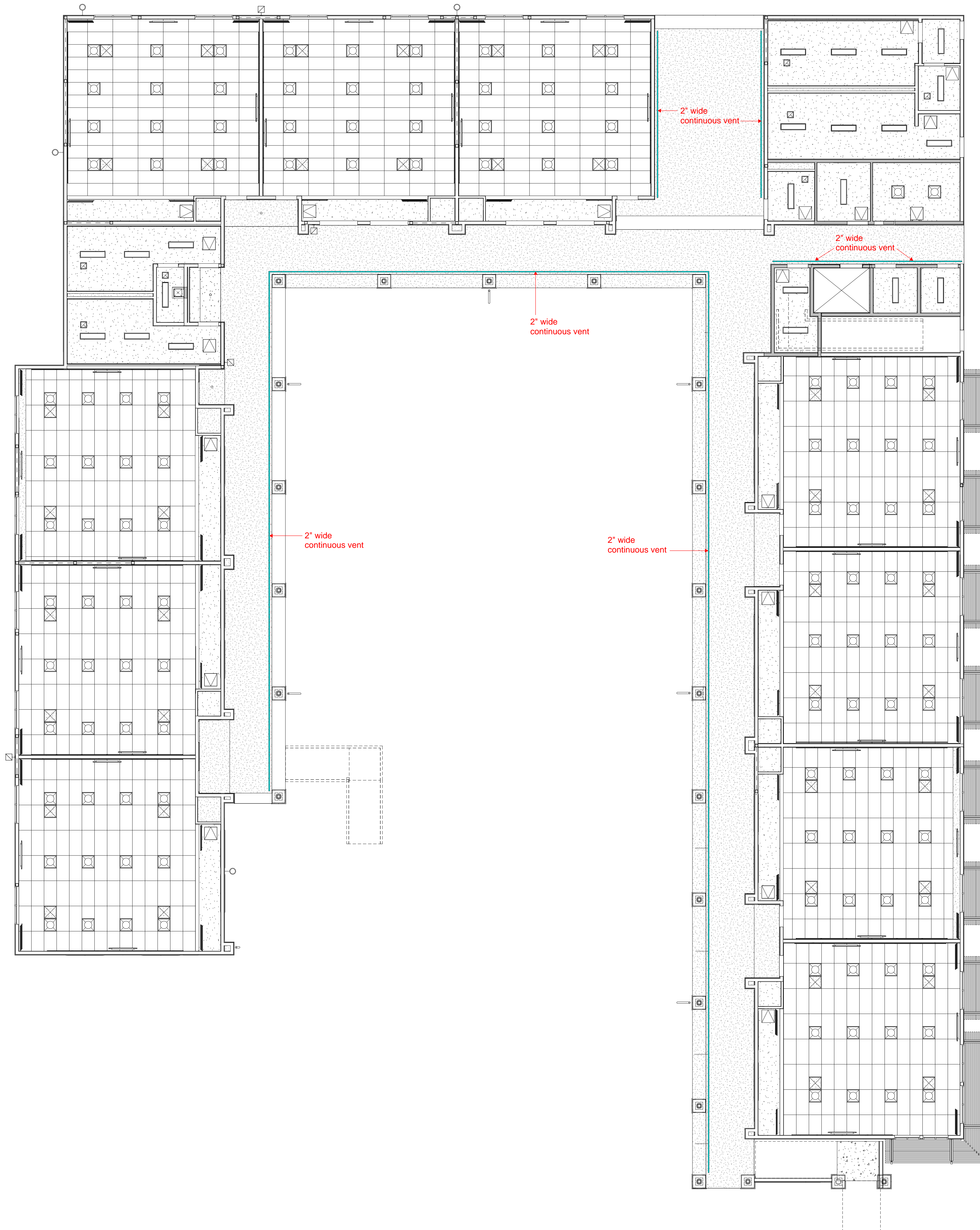
CLASSROOM - FIRST FLOOR SOFFIT VENTING
