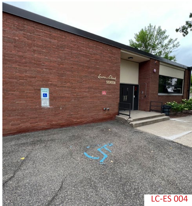
Accessible parking spots are located next to a non-accessible building entrance.
