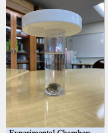
Experimental Chamber: Measured metabolic rate determined by oxygen consumption
