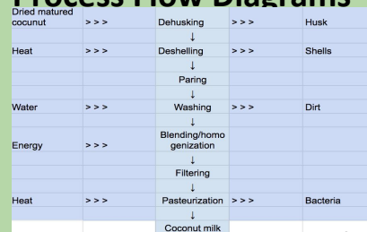
Figure 2: Process flow diagram for coconut milk
