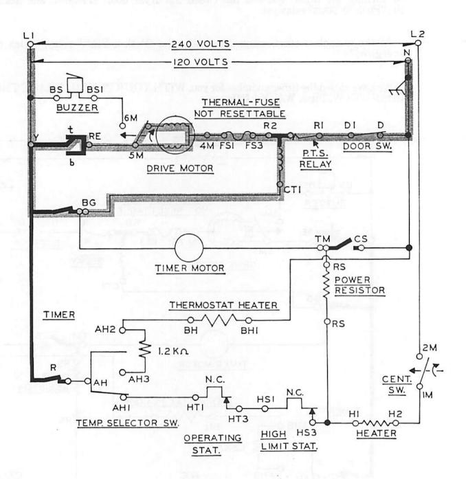
The wiring diagram on this page shows the circuits that are made with the dryer running in the "REGULAR" cycle. We have closed the proper switches for this condition for you.
