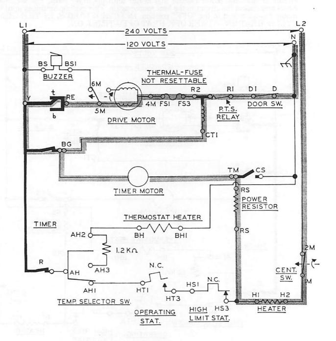
With 5 minutes left at the end of the "REGULAR" cycle, timer switches Y-R open and TM-CS close. Timer contact Y-RE(T) opens the circuit to the drive motor and allows a momentary circuit to be completed through the buzzer and run windings of the drive motor. As the motor slows down, centrifugal switch 5M to 6M opens. This opens the buzzer circuit causing it to stop buzzing.
