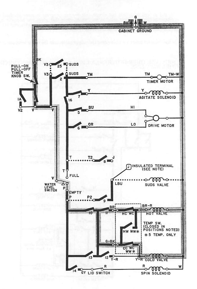
Very good! In the last diagram the washer was filling with water. By looking at the response you can see that neither the main drive motor, agitate solenoid nor the timer motor circuits were energized. In the diagram below the water level switch has moved to the FULL position because the washer has filled with water. The same timer switches that were closed in the last diagram are closed. We have closed them for you. DRAW A WAVY LINE THROUGH THE ENERGIZED CIRCUITS.
