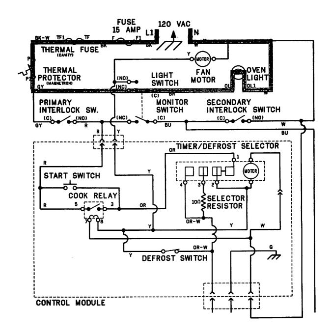
Great! Now with the door shut, turn the microwave "ON." TRACE THE ACTIVE CIRCUITS WITH A WAVY LINE.
