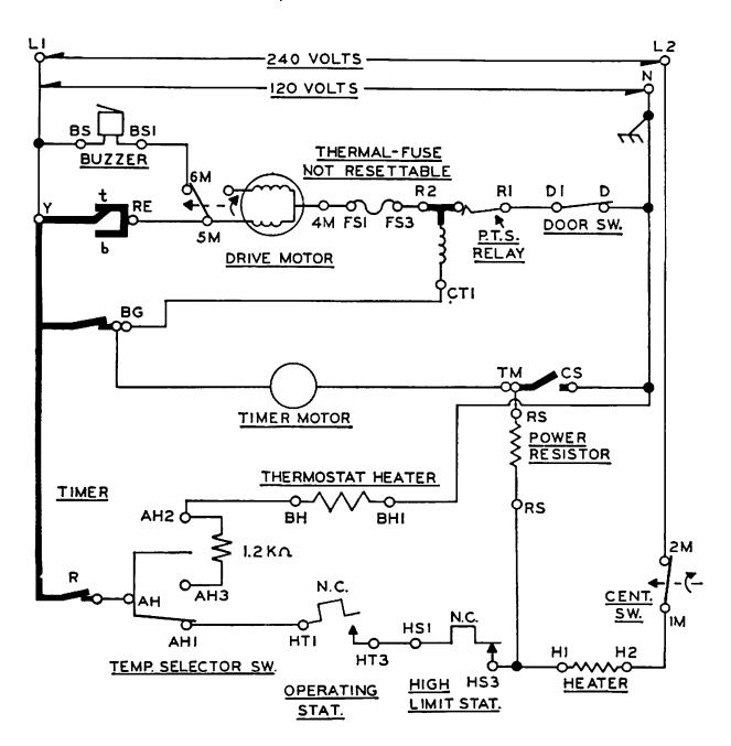
TRACE THE ACTIVE CIRCUITS BY DRAWING A WAVY LINE THROUGH THEM.
