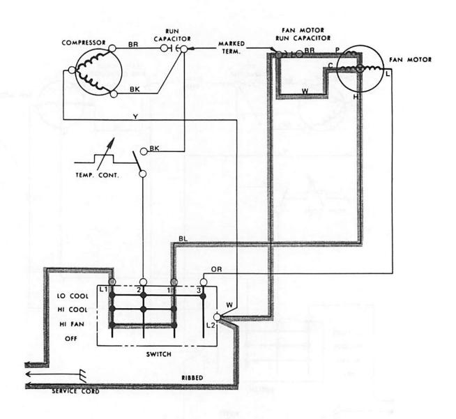
The fan circuit in the HI COOL and the HI FAN positions will be the same. Remember that this air conditioner temperature control switch (thermostat) closes on heat rise.
