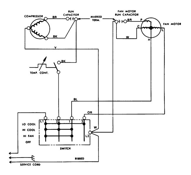
NOTE THAT NEITHER THE COMPRESSOR NOR THE FAN MOTOR USES A STARTING RELAY. THESE MOTORS ARE OF THE PSC (permanent split capacitor) TYPE.
