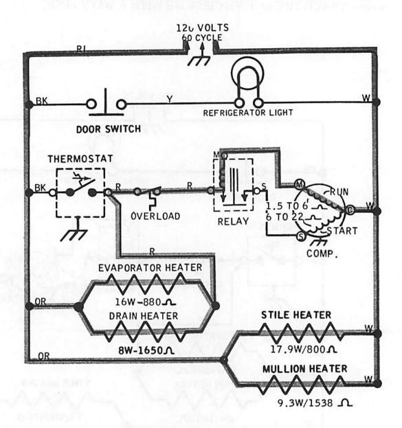
The parallel evaporator-drain heater circuit is now active. Although current is flowing through the relay coil and the compressor run winding, there is not enough current to energize the start relay and run the compressor.
