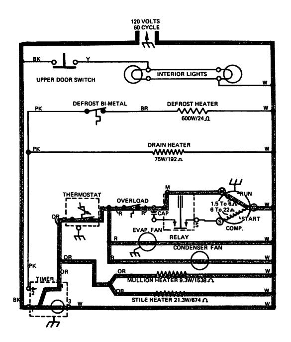
Note the defrost timer in this diagram. It has closed to contact number 2 and the refrigerator is now defrosting. TRACE THE ACTIVE CIRCUITS WITH A WAVY LINE.
