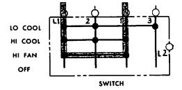
If the switch is set on HI COOL, the circuit through the switch is: (You draw this one.)
