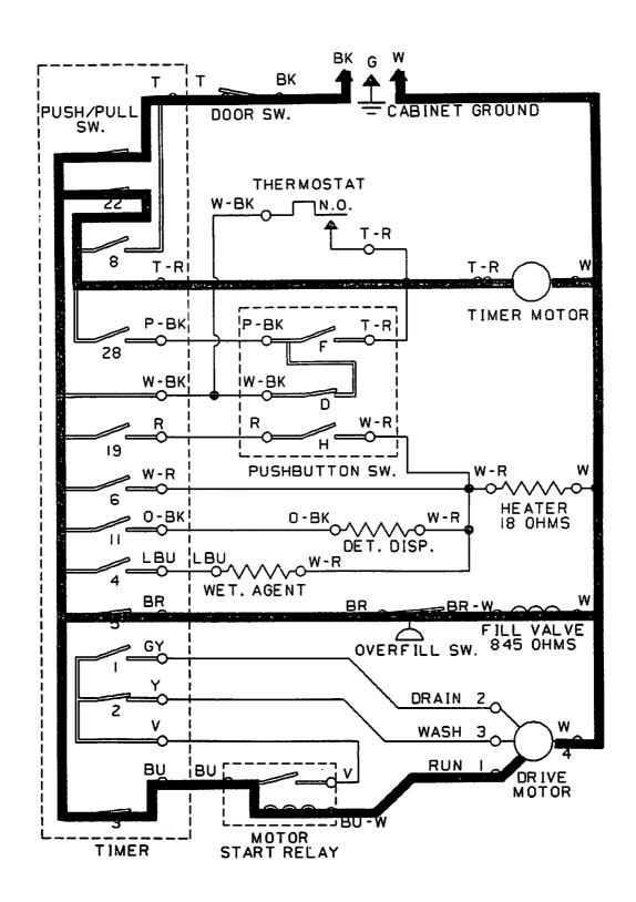
Let's trace the circuits for a "heat dry" cycle. During this cycle the drive motor stops running and timer switches 1, 19 and 22 are closed. Once again, we have closed the contact in the pushbutton selector switch and the push/pull switch for you.
