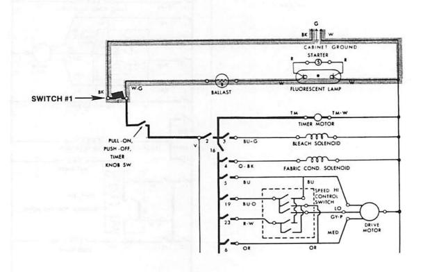
You did so well with that last circuit that we can progress to more involved circuits. Let's assume that you have selected the "wash" cycle that gives you hi-motor agitaiton, your water temperature, and have started the washer. The timer has advanced to a position where it has closed timer switches 1, 5, 7, 10, 11 and 16.
