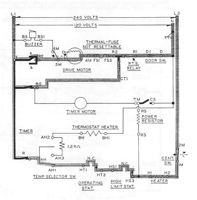
Did you show the buzzer circuit as an active circuit? Remember, it is a basic principle of electricity that current will always follow the path of least resistance. In this case the current bypassed the buzzer circuit and flowed through timer contacts Y-BG and the drive motor circuit—a line of least reistance.
