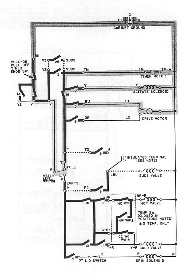
You are doing very well! Now let's suppose the timer has advanced and closed timer switches 1, 2, 5, 14 and 16. The LID SWITCH is also closed because the lid is shut. This puts the washer in the SPIN cycle. We have closed the switch contacts in the water temperature switch for you as we have done in the past diagrams.
