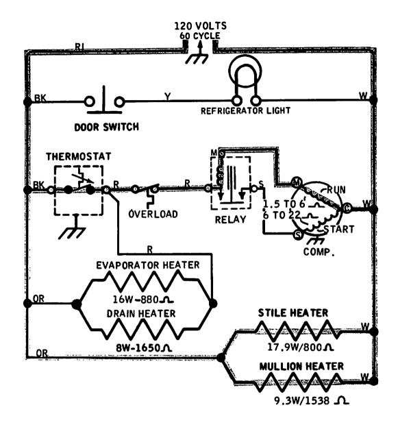
Did you show the parallel circuit for the evaporator heater and drain heater as an active circuit? One of the basic principles of electricity is that current will always follow the path of least resistance. In this case the current bypassed the parallel evaporator-drain heater circuit and flowed through the thermostat contacts, a line of least resistance, and on to the compressor.
