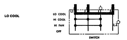
Now that you know how to trace a circuit through the air conditioner switch, we want you to trace out a complete circuit.
