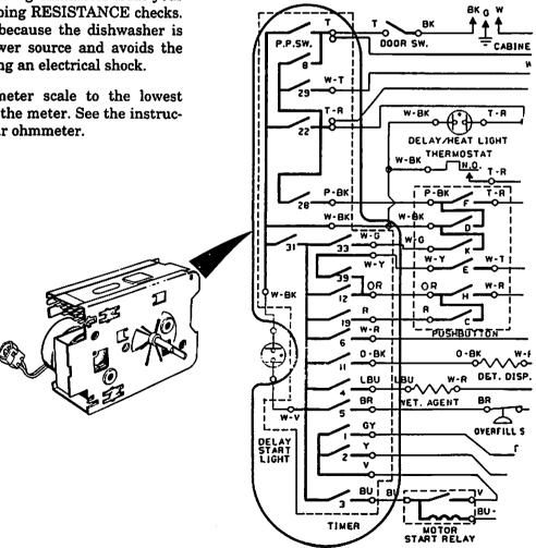
STEP 7 EXAMPLE: Move the timer to the start of NORMAL wash. PROBLEM: Dishwasher does not fill.
