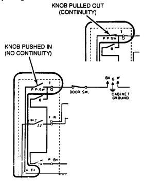
STEP 11 If the door switch is good but the dishwasher still won't start when the timer knob is pulled out, check the internal timer push/pull switch (P.P.SW.) contacts.
