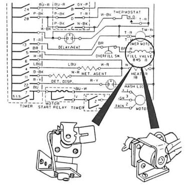
STEP 2 Refer to the instructions that came with your ohmmeter to find the proper scale to measure 500 to 2,000 ohms. Set the ohms scale and ZERO the meter.
