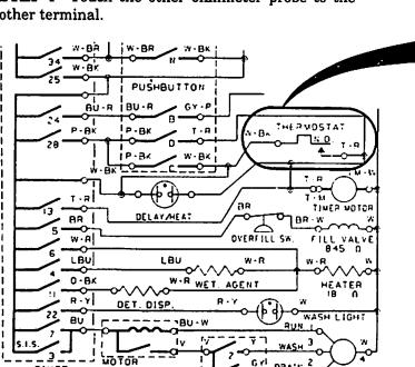
STEP 5 The ohmmeter should show an open circuit. If not, the thermostat is bad and needs replacing.
