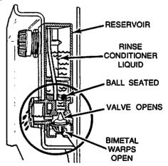
During the final rinse, current flows to the bimetal heater. This causes it to warp downward. The valve opens and a small amount of wetting agent (approximately 1 cc or .03 oz.) flows into the dishwasher.
