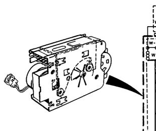
STEP 9 Touch one ohmmeter probe to terminal T.
