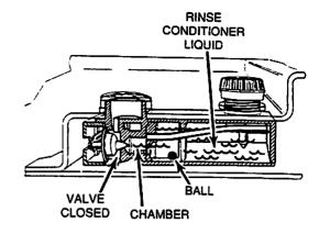
When the door is opened for loading, the wetting agent flows into the dispensing chamber because the sealing ball has fallen away from its sealing position.
