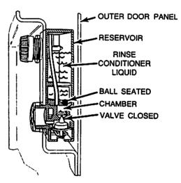
when the door is closed, the sealing ball rolls back into its sealing position and seals the now full dispensing chamber.
