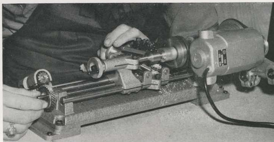
PRECISION TURNINGS, accurate to .0005 inch, can be crafted by this lathe.
