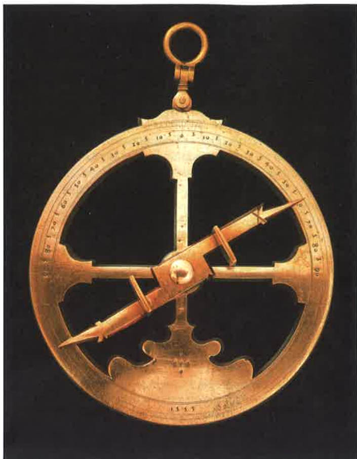
Portuguese Mariner's Astrolabe, 1555 Between 1500 and 1635 over nine hundred ships sailed from Portugal to ports on the Indian Ocean, in annual fleets composed of five to ten ships. Portuguese sailors used astrolabes, such as the bronze example shown here, to accurately plot their position. (Granger/Granger — All rights reserved)
