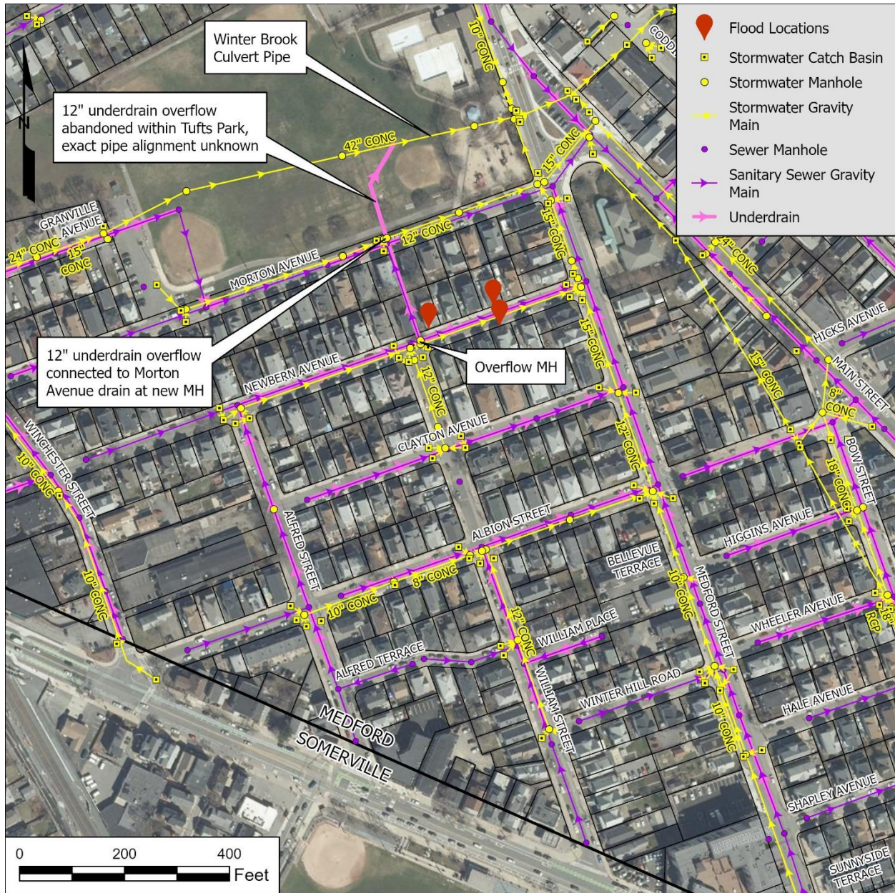
Figure 6: Newbern Avenue underdrain connection
