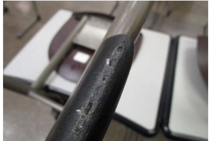
CLOSE UP OF DIRT EMBEDDED IN PLASTIC FOOT PAD
