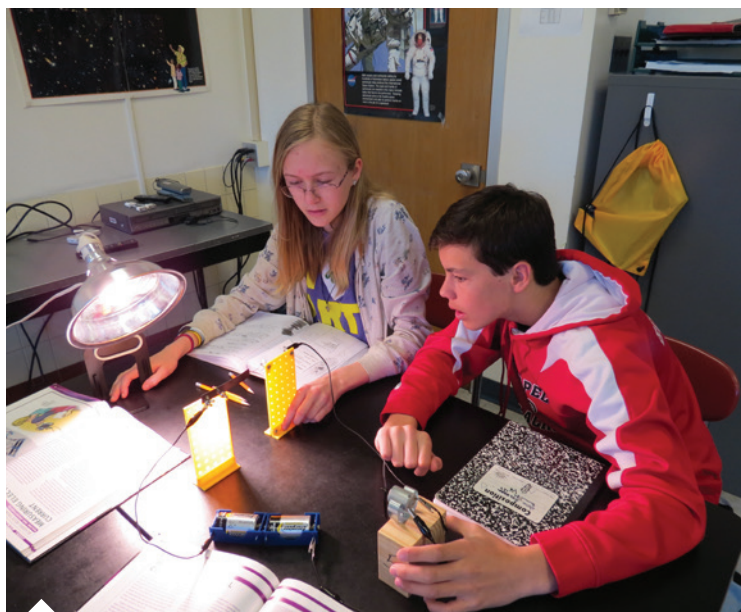
Students examine a closed electrical circuit. When the light hits the bimetallic strip, the strip bends and forces the fan to turn on. As the fan cools the strip, the fan turns off. The students can move the light closer or farther away to view the different reactions.
