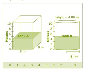
Volume of Tank A is:  $8m \times 8m \times 4m = 256m^3$
