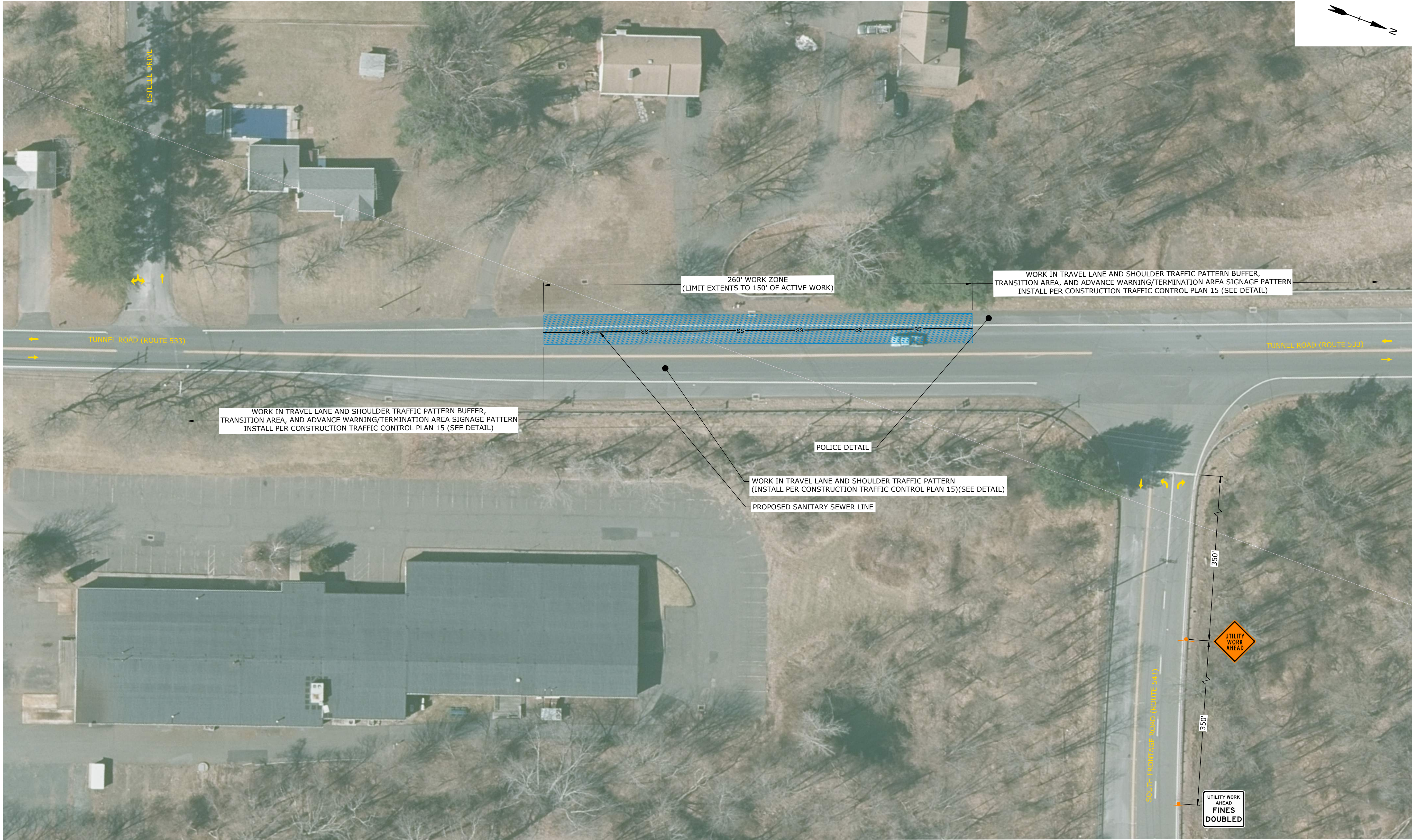
EXIT 66 SEWER EXTENSION TEMPORARY TRAFFIC CONTROL PLAN - PHASE 2 (MON-FRI, 9AM - 4PM)
