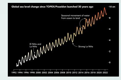
Global sea level change recorded by satellites TOPEX-Poseidon, Jason-1, Jason-2, and Jason-3.
