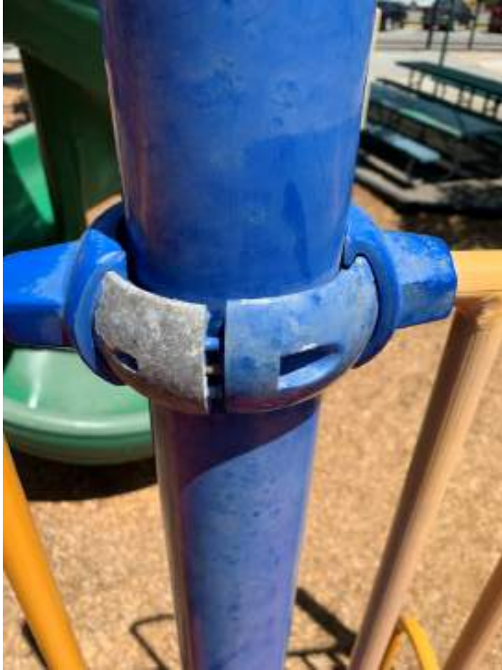
Support Clamps broken and pulling apart.
