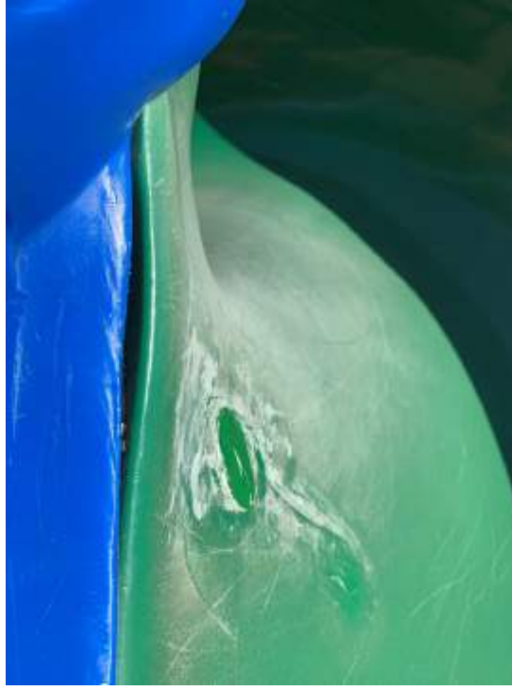
Entanglement Hazard at spiral slide entry.
