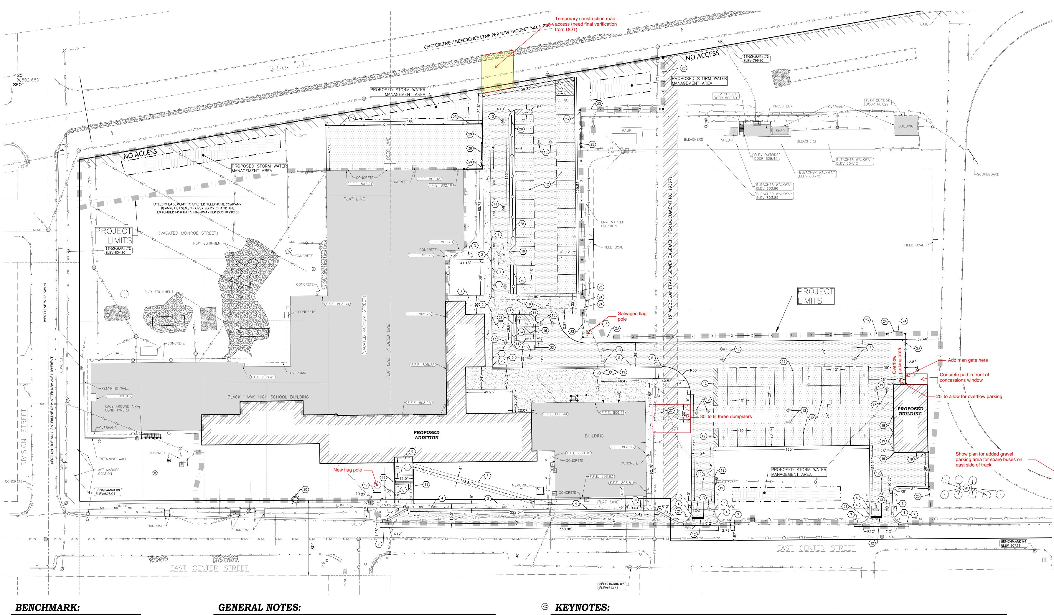
ELEVATIONS ARE REFERENCED TO NAVD 88 DATUM. BENCHMARK #1 NORTHEAST FLANGE BOLT ON HYDRANT LOCATED AT THE NORTHEAST CORNER OF THE INTERSECTION OF DIVISION STREET AND EAST CENTER STREET.
