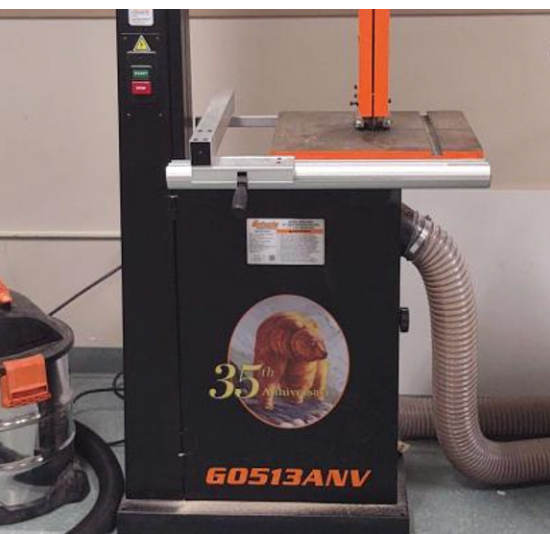
A bandsaw used by engineering students to cut wood and plastic.
