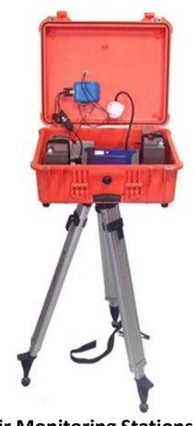
Air Monitoring Stations (with telemetry)
