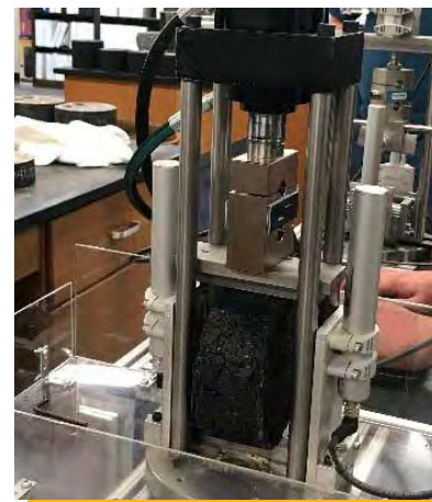
Image Source: FHWA Load Frame performing Ideal-CT
