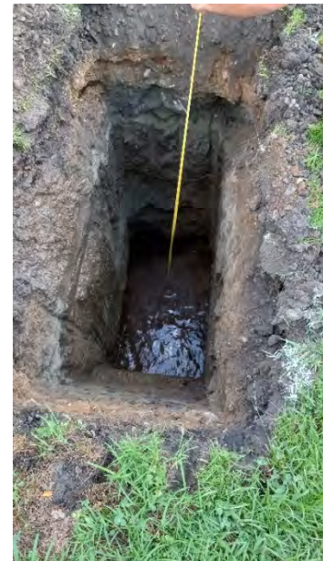
Short-term equilibrium groundwater level measured at approximately 6.5 feet below ground surfaces
