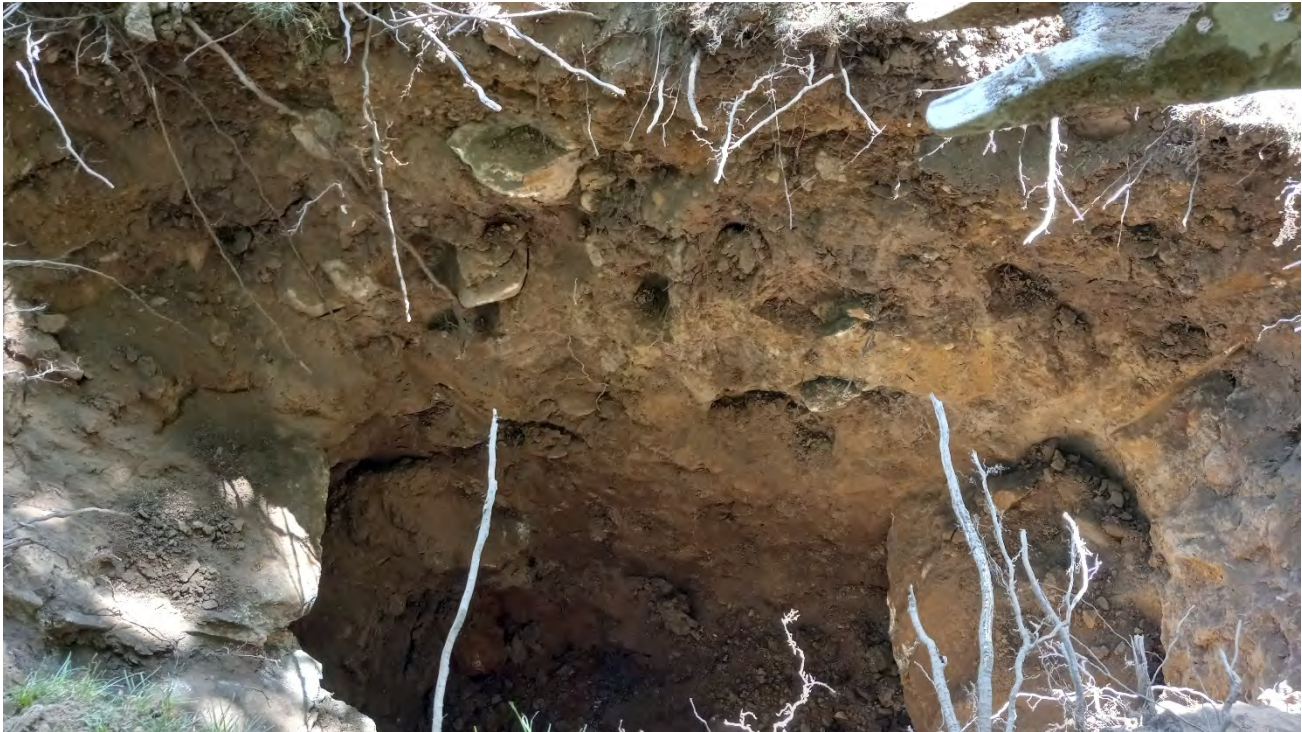
In progress TP-04. – Short-term equilibrium groundwater level measured at approximately 8 feet below ground surfaces
