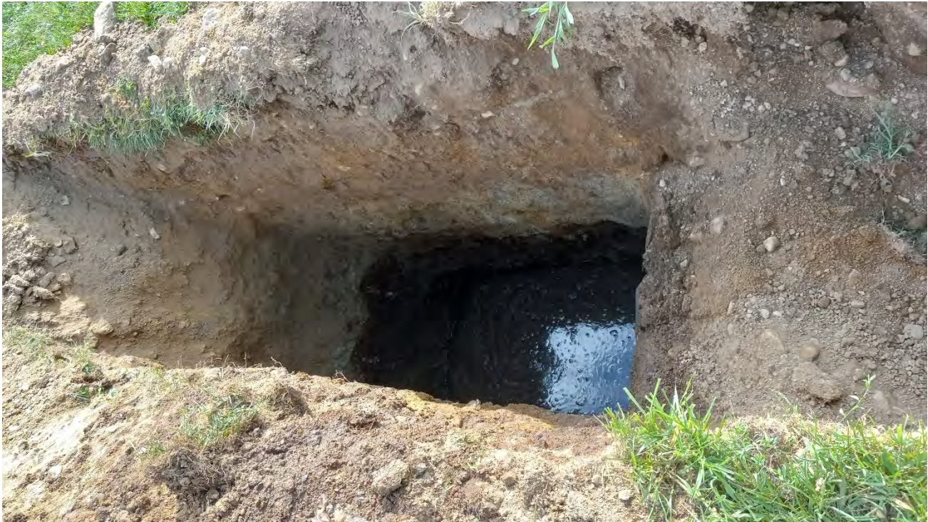
In progress TP-02. – Short-term equilibrium groundwater level measured at approximately 6.5 feet below ground surfaces
