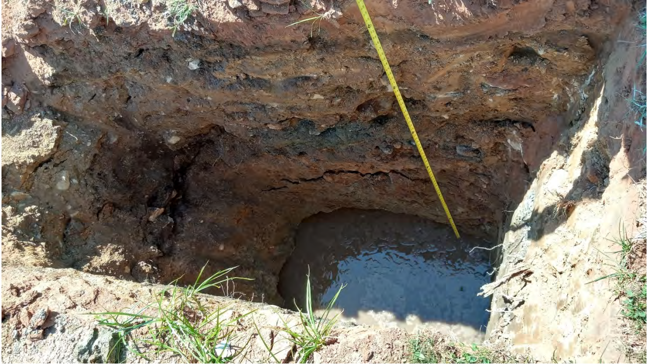
In progress TP-06. – Short-term equilibrium groundwater level measured at approximately 7.5 feet below ground surfaces
