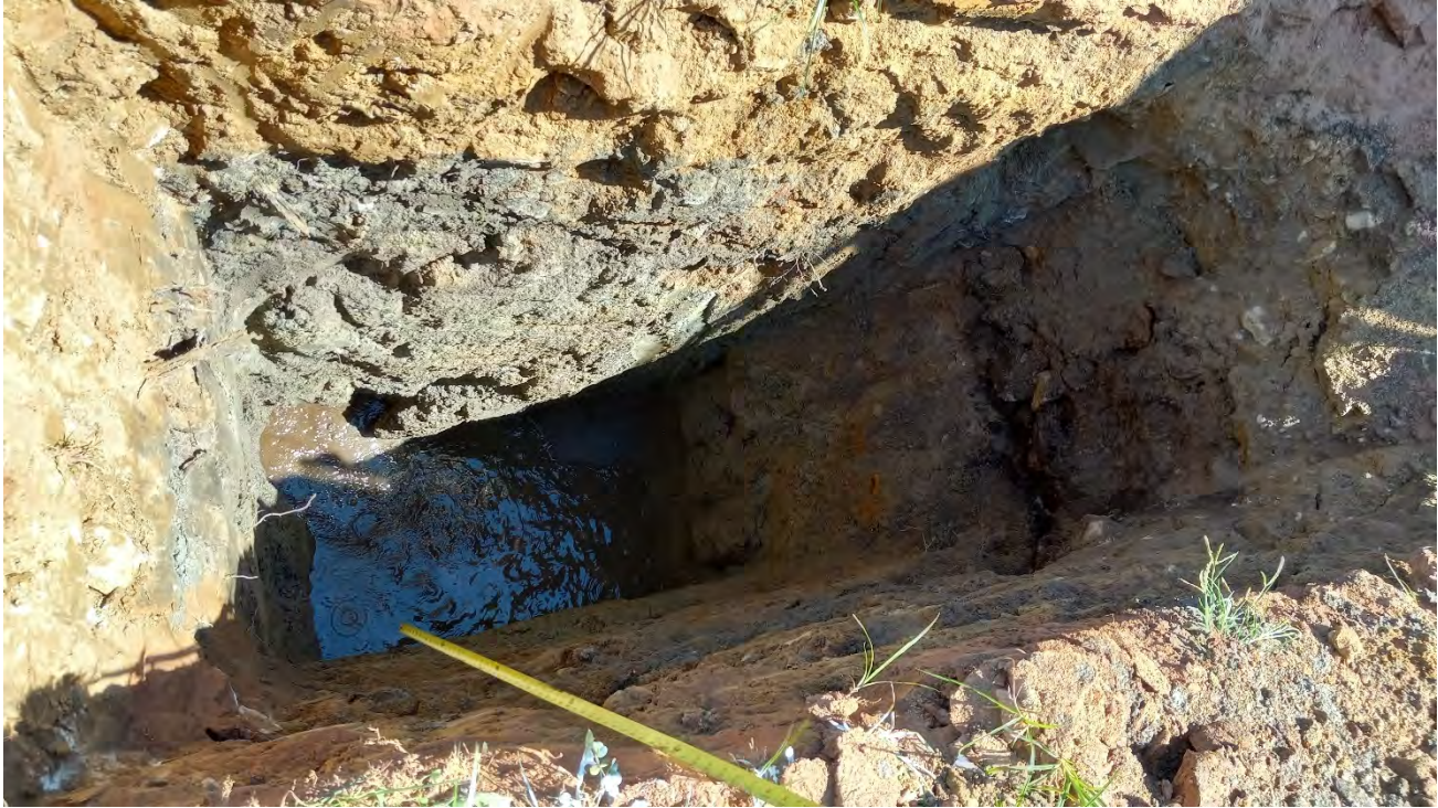
In progress TP-05. – Short-term equilibrium groundwater level measured at approximately 6.2 feet below ground surfaces
