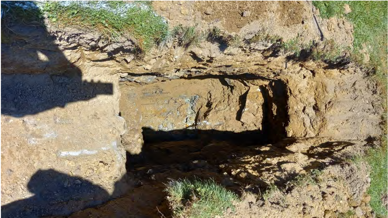
In progress TP-07. – Short-term equilibrium groundwater level measured at approximately 9.5 feet below ground surfaces
