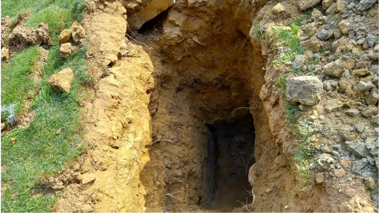
In progress TP-11. – Short-term equilibrium groundwater level measured at approximately 9.0 feet below ground surfaces
