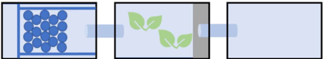
Figure 2. Top view of constructed wetland. Tube settlers angled at 60° to settle out suspended solids and decrease the amount of settling area needed.
