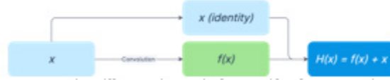
Figure 5. An illustration of the residual connections of ResNet. The identity of the initial function, x , is added to the feature map after convolution, f(x) , to produce the output.
