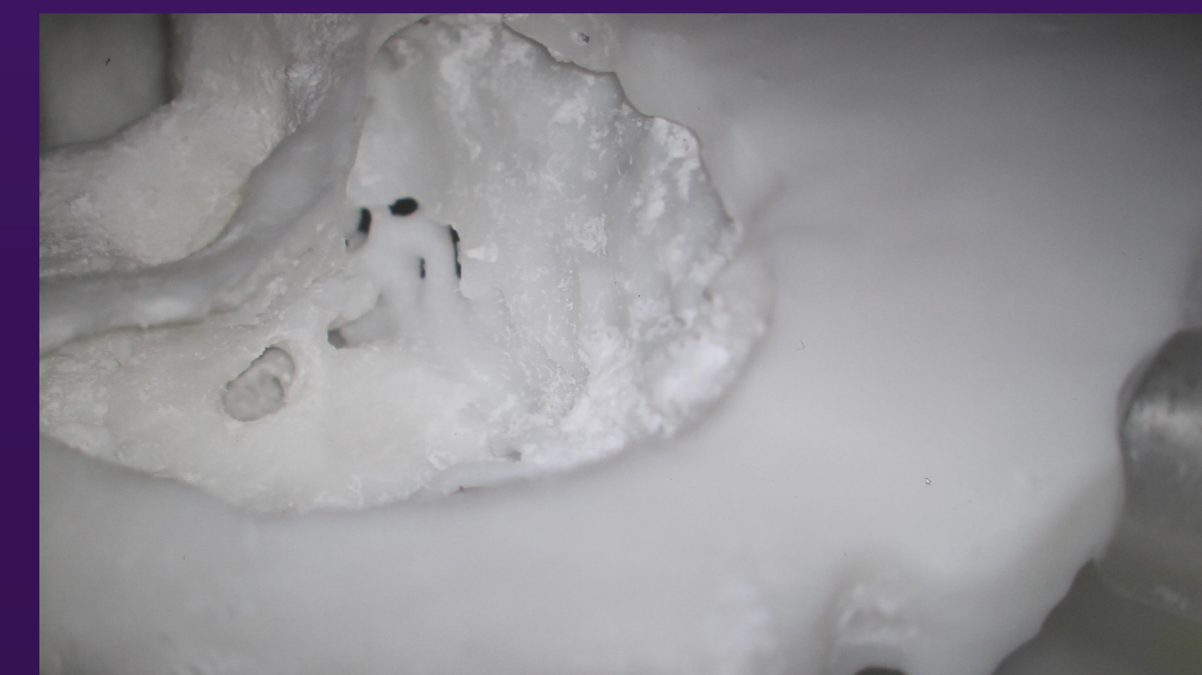
Figure 4: Microscopic image of the 3D printed temporal bone made with Formlabs resin. Image shows the middle ear bones after drilling the model.
