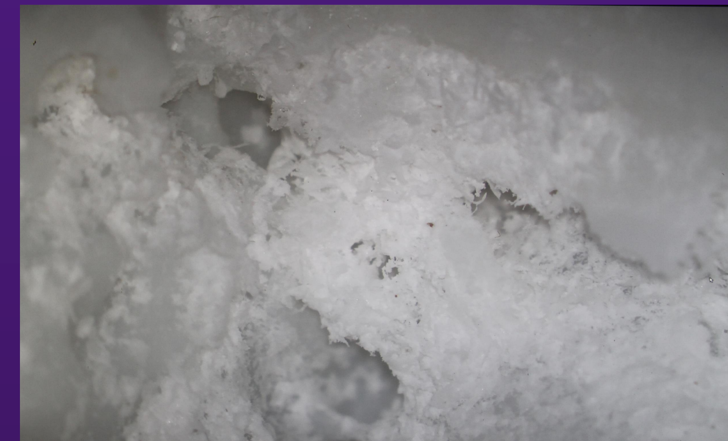
Figure 3: Microscopic image of the 3D printed temporal bone made with Formlabs resin. Image shows the dust created after drilling the model.
