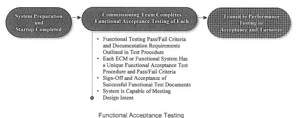
Functional acceptance testing will vary greatly for each of the ESMs and each of the systems within the ESMs. Actual tasks for each of the ESMs and systems (chilled water systems, steam systems, energy management controls system, photovoltaic systems) will be included in functional acceptance test forms generated for that specific ESM or system.
