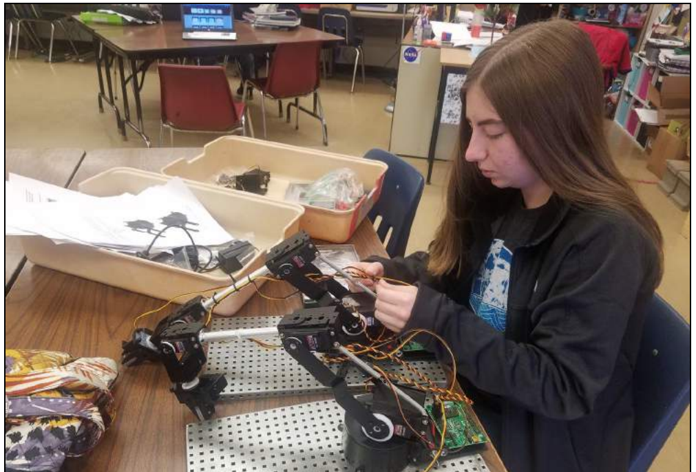
Computer Integrated Manufacturing student, Hannah works on two robotic arms using one as a model to troubleshoot the other.
