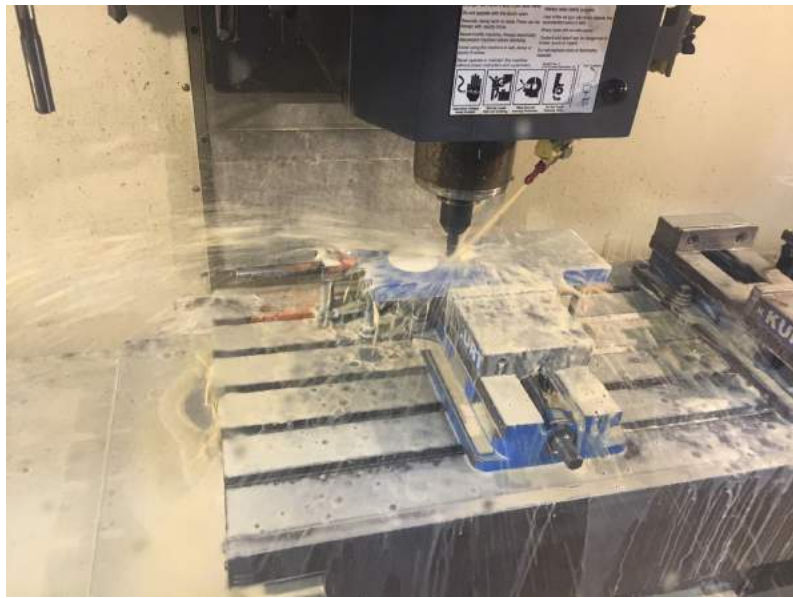
We were able to watch the plaque being cut from billet aluminum on a Haus CNC machine using G Code similar to what runs our 3D printers.
