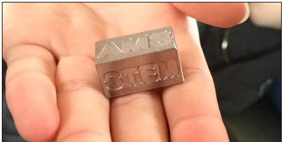
Mini STEM block programmed and CNC cut out of billet aluminum.
