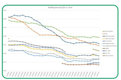
Cost intensity is the sum of what an entity is billed for electric and gas cost for the 12-month period prior to the year ending date, all divided by the square footage of the building. In the graphics shown here, since 2014 Northmont has drastically decreased cost intensity through energy saving projects implemented through the Strategic Plan.
