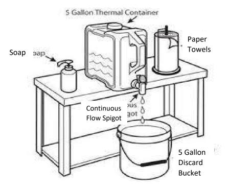
The temporary handwashing station shall consist of at least a 5-gallon insulated container with spigot that provides continuos flow of warm (100°F-120°F) running water, soap paper towels, a reminder sign, a 5-gallon bucket to collect the wastewater, and a trash container to discard wastepaper.
