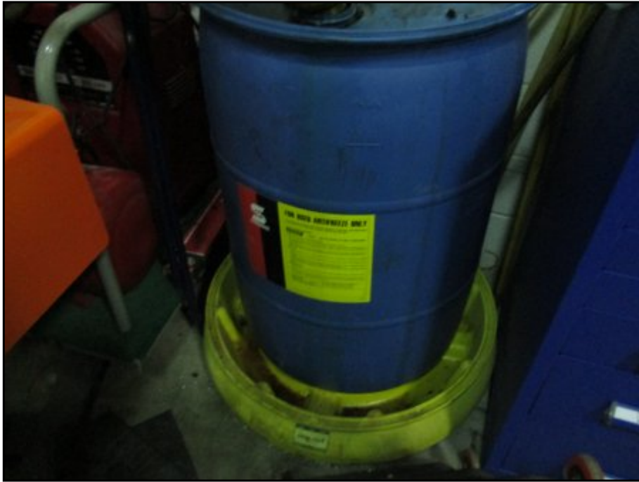
View of the 55-gallon drum of used anti-freeze in secondary containment in the autoshop of the main building on the Property.
