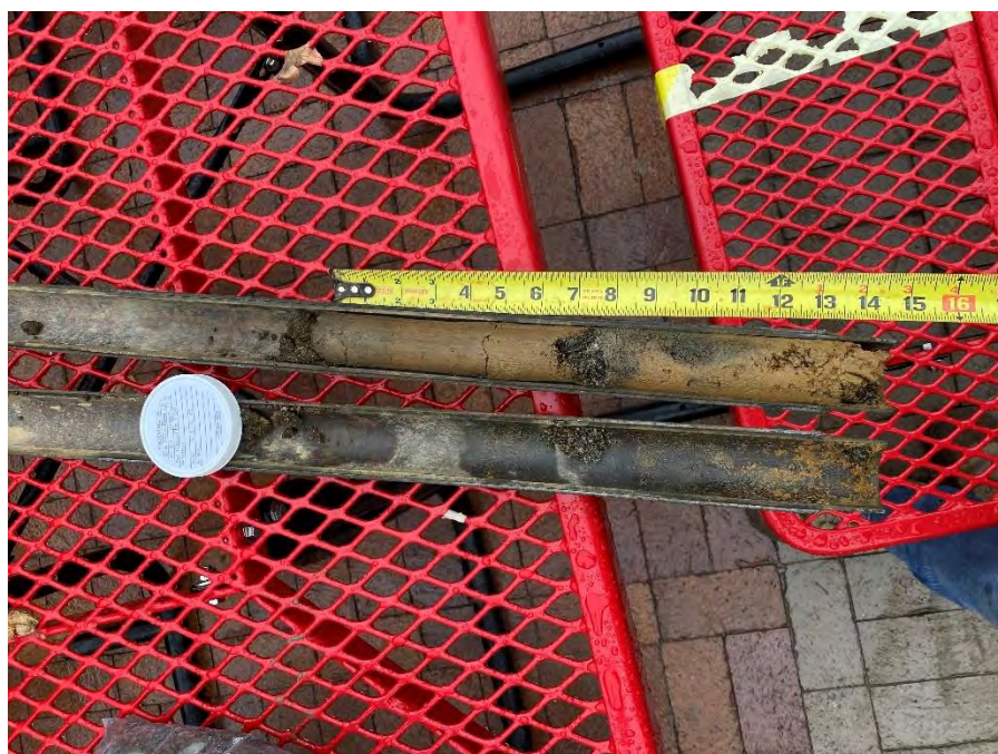
Photo 6: Silt layer from boring LB-01
