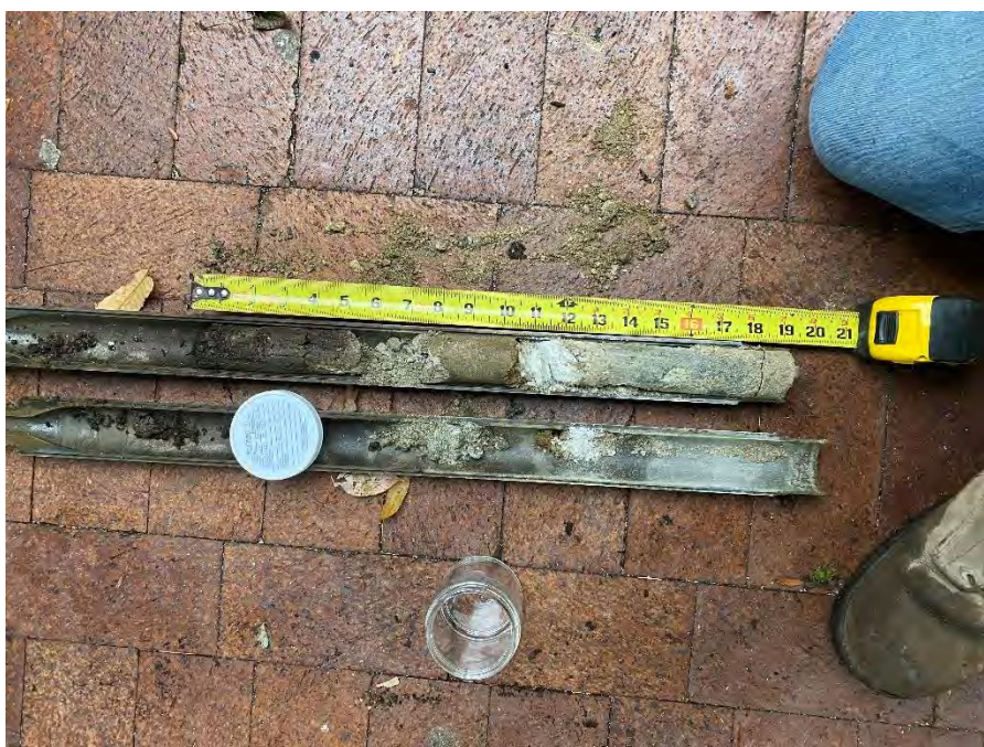
Photo 4: Typical transition from fill to native sand layer from boring LB-03
