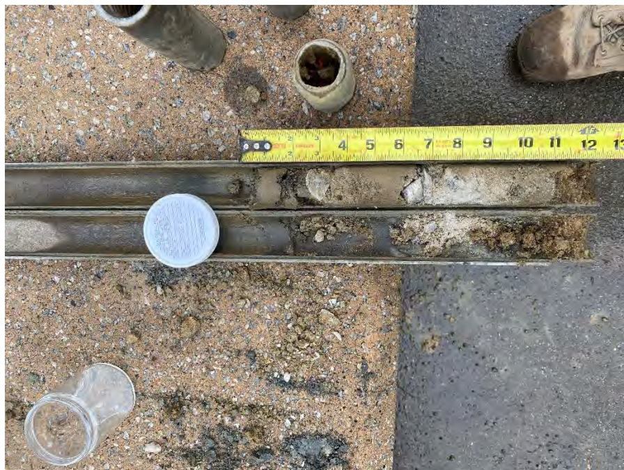
Photo 5: Decomposed rock from boring LB-02.
