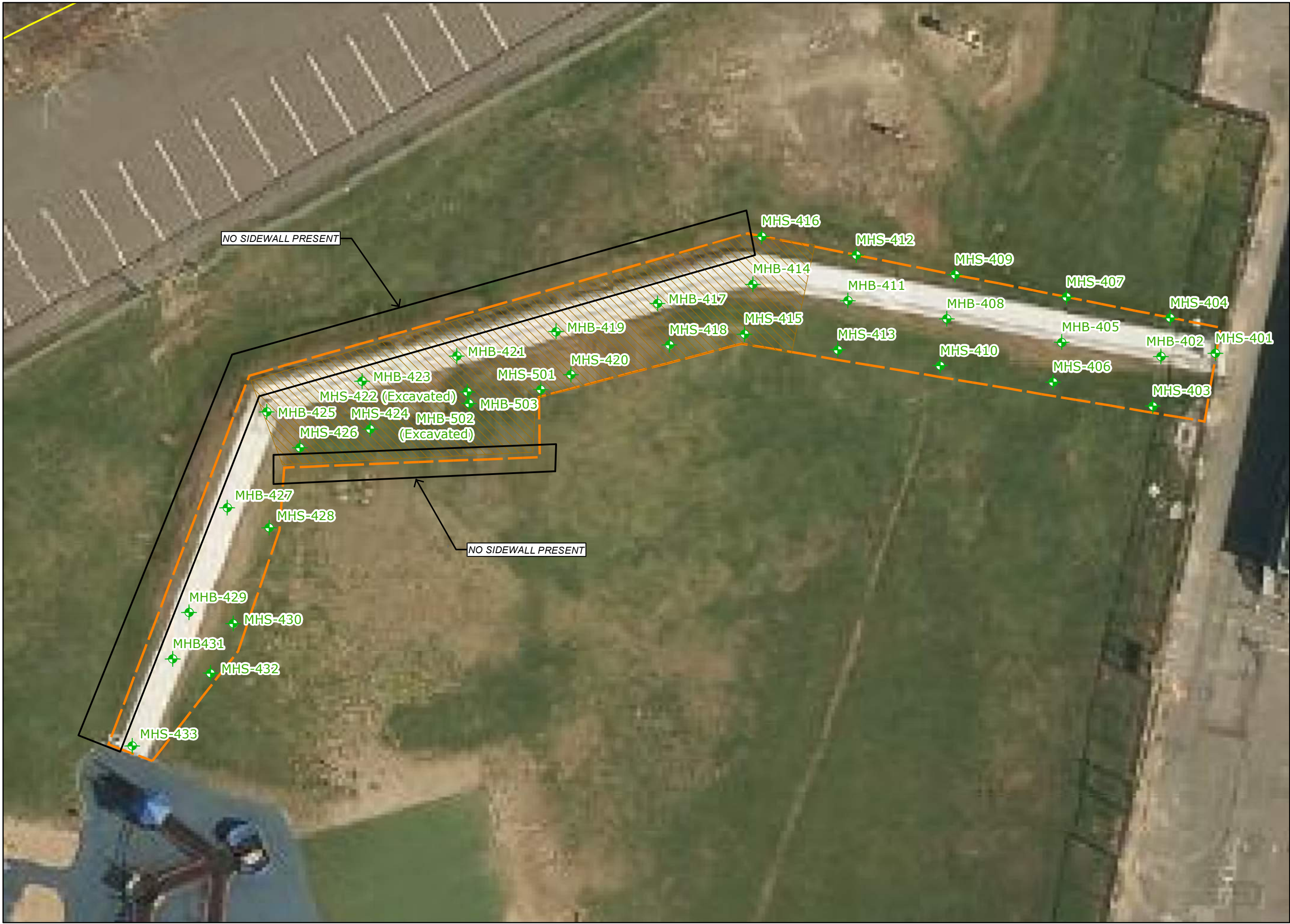
FIGURE 6 FINAL EXCAVATION LIMITS & ENDPOINT SAMPLE LOCATIONS
