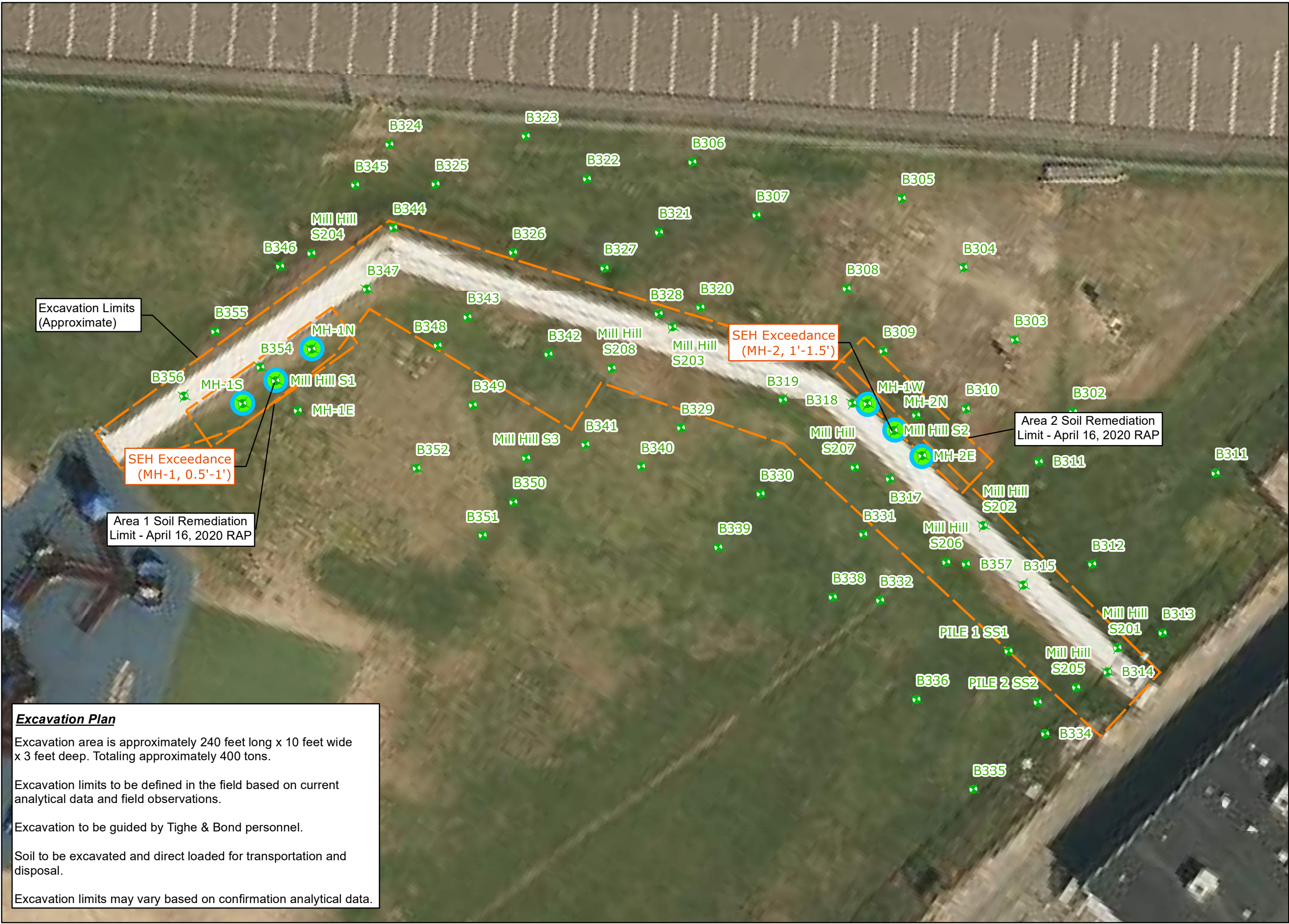
FIGURE 5 PRE-REMEDIALTION SOIL EXCAVATION PLAN
