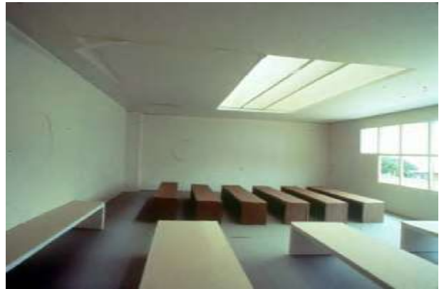
Physical model to study daylighting
