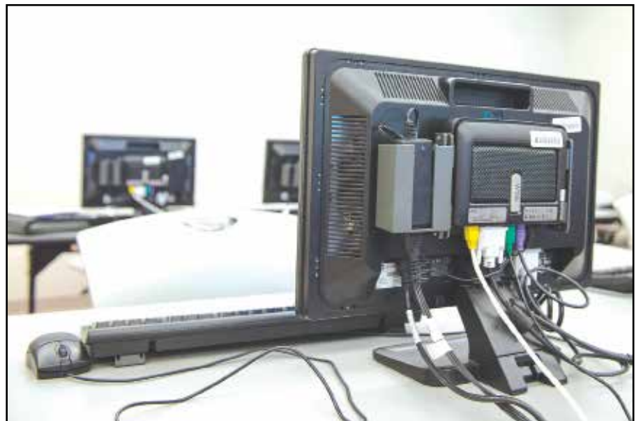
The thin client is attached to the back of the monitor..
