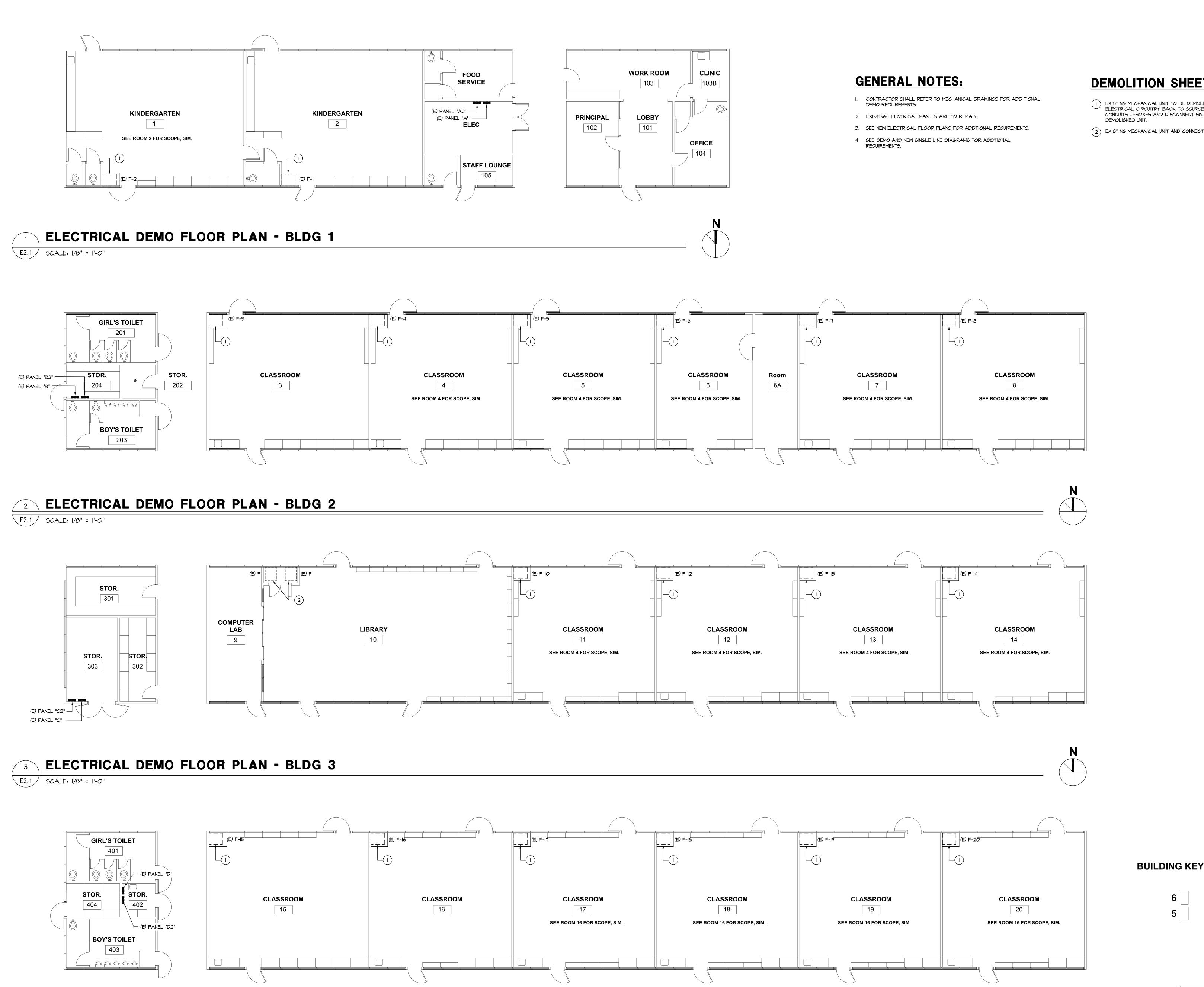
**DEMOLITION SHEET NOTES:** EXISTING MECHANICAL UNIT TO BE DEMOLISHED. PULL EXISTING ELECTRICAL CIRCUITRY BACK TO SOURCE AND REMOVE. REMOVE ALL CONDUITS, J-BOXES AND DISCONNECT SWITCH ASSOCIATED WITH THE (2) EXISTING MECHANICAL UNIT AND CONNECTIONS TO REMAIN.
