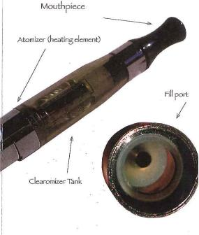
An atomizer generally consists of a small heating element responsible for vaporizing liquid, and a wicking material that draws liquid in. Along with a battery, the atomizer is the central component of every personal vaporizer. Once vaporized, the liquid/solution is odorless and invisible, however, other problems may be coming to light.
