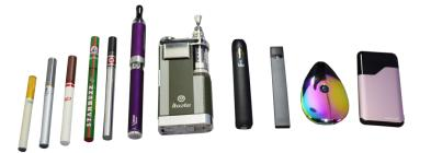
E-cigarettes come in many shapes and sizes. Most have a battery, a heating element, and a place to hold a liquid.
