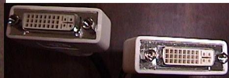
Dual VGA and DVI Video card connectors
