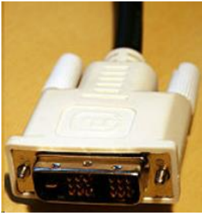
Monitor DVI Cable (Digital Video Input)
