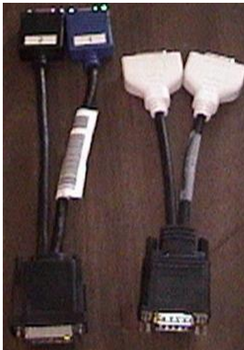
Dual VGA and DVI Video card connectors
