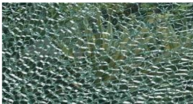
Tempered glass breaking pattern
