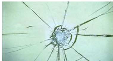
Laminated glass breaking pattern
