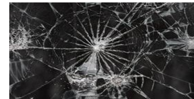
Glass with security film breaking pattern
