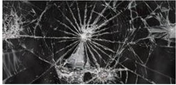
Glass with security film breaking pattern
