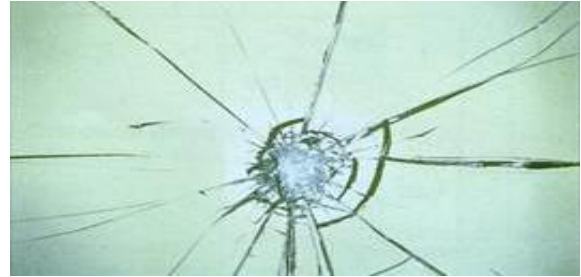
Laminated glass breaking pattern
