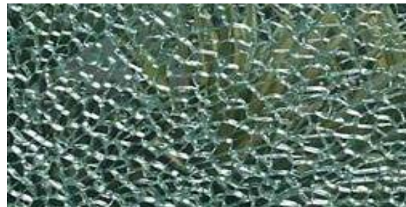
Tempered glass breaking pattern
