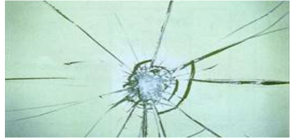
Laminated glass breaking pattern
