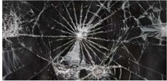
Glass with security film breaking pattern
