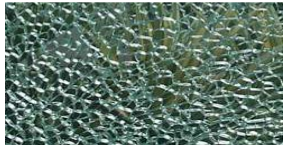
Tempered glass breaking pattern
