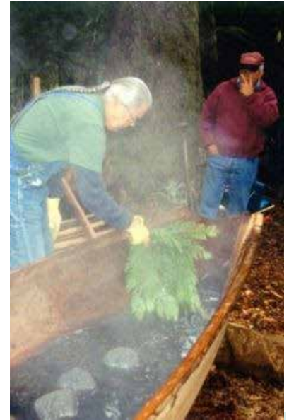
Brothers Gary Johnson (left) and Leroy Johnson steam the traditionally constructed canoe built by Tony Johnson for Fort Clatsop. They are following the steps their ancestors took to make canoes. In 2022, Gary and Tony were members of the Chinook Indian Nation Council.
