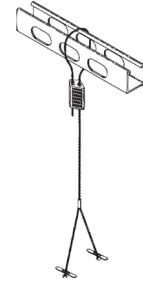
HB-XX-18Y-PAD Y-Toggle Cable System (xx = in)
