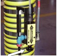
Activate the "Black" button on the system valve to pressurize the "Grabber" boot which works like a mechanical seal for the system.
