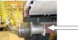
Place the "Grabber" boot over the vehicle exhaust adaptor up to the stop disk
