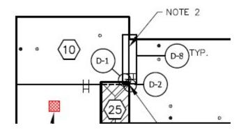
NOTE 2: THREE (3) COURSES OF BRICK TO BE REMOVED ABOVE EXISTING TERMINATION BAR ALONG ENTIRE WALL LENGTH TO INSTALL NEW THROUGH-WALL FLASHING AND SHEET METAL (APPROXIMATELY 20 LF). MASONRY TO BE REINSTALLED OVER NEW THROUGH-WALL FLASHING AND SHEET METAL PER DETAIL D-8.
