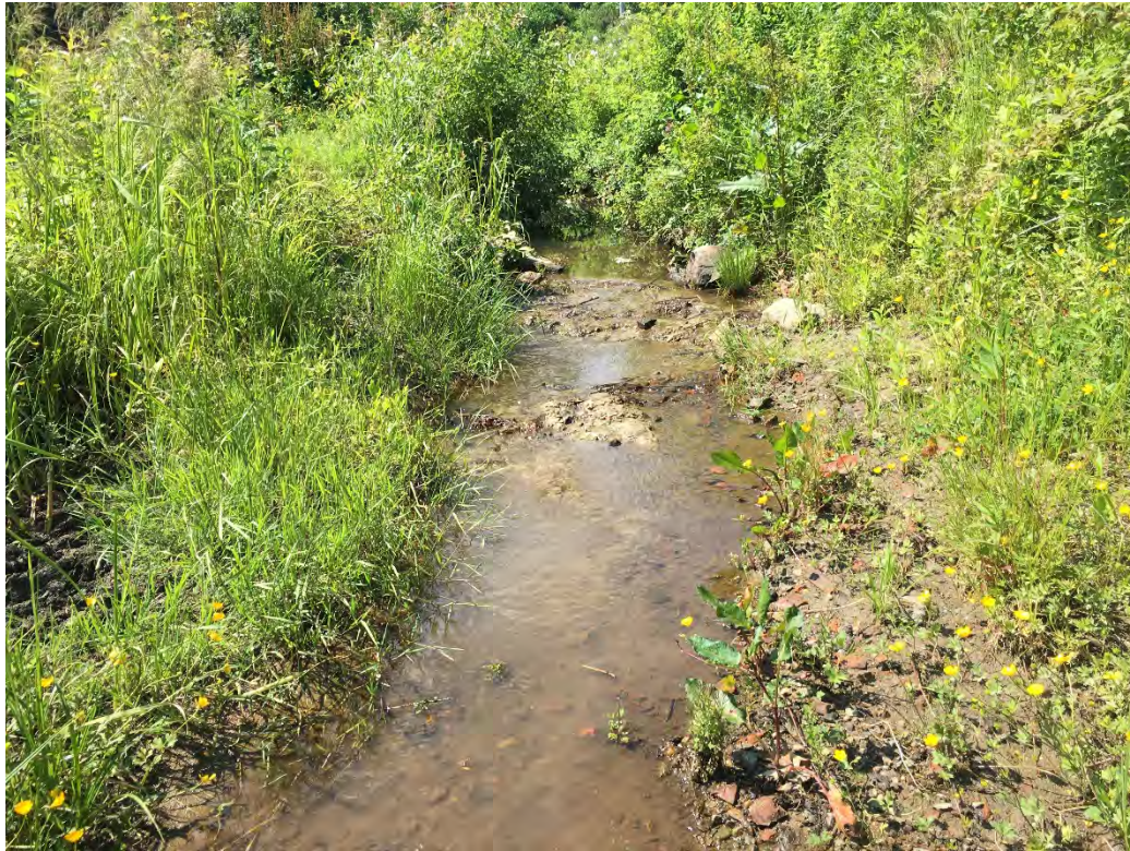
Photo 1: Phillips Bk with bank conditions with a BEHI rating of Very Low
